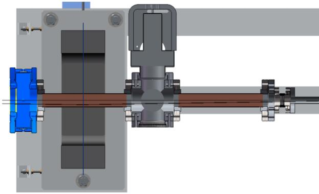
Figure 2. Injection Chicane top cut view with electron beam and laser path shown.
