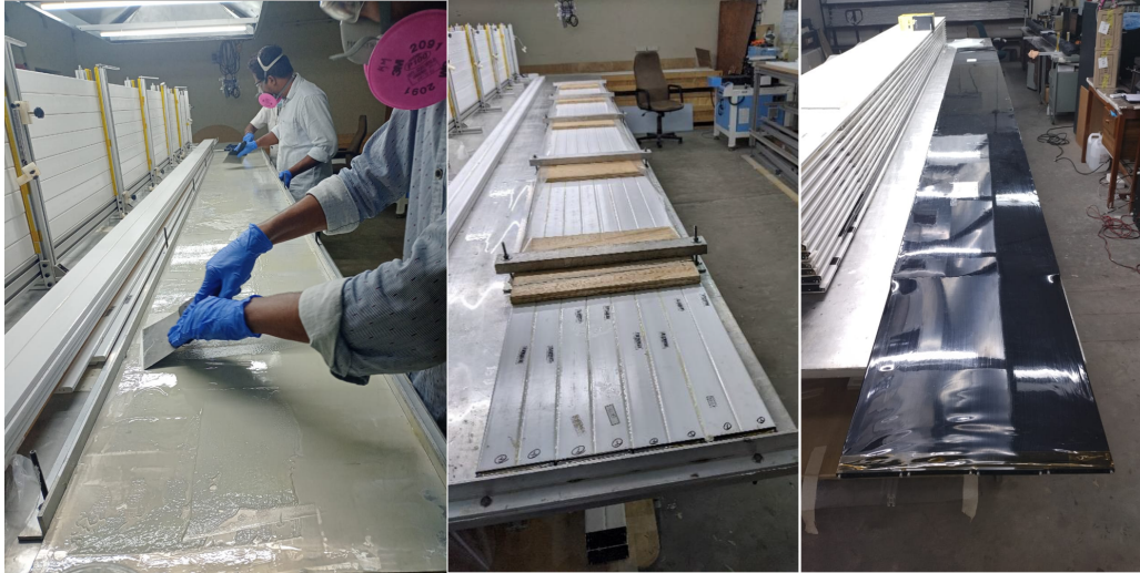
Figure 3: Various steps involved in the production of di-counters and detector tile assemblies.
