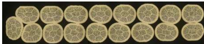
Fig. 1. Bi2212 Rutherford cable cross-section [4].
