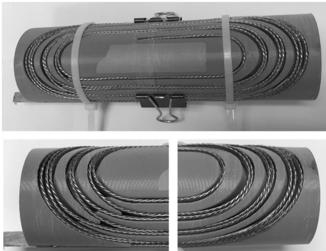
Fig. 6. Single-layer plastic half-coil (top) and practice half-coil LE (bottom left) and non-LE (bottom right) views. One can see the short inter-block cable transitions in the LE on the bottom left picture. The size of coil end blocks needs to be optimized to minimize the gaps between turns and structure.
