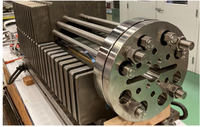
Fig. 9. SMCT coil end support system.
