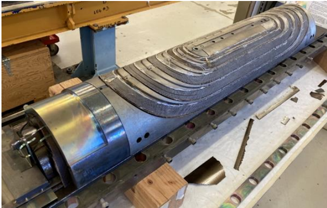
Fig. 3. SMCT coil after reaction. As expected, the space for the cable expansion reduced (but not eliminated). No insulation damage during reaction was found.
