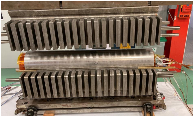
Fig. 8. Coil assembly covered by the protection shell is being enclosed by the top part of the yoke.
