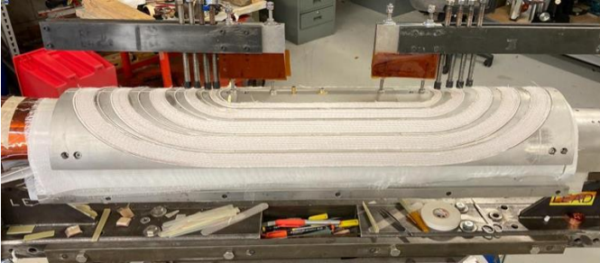
Fig. 2. SMCT coil after winding into SM structure. The space in blocks for cable transverse expansion simplifies insertion of last turns in blocks.
