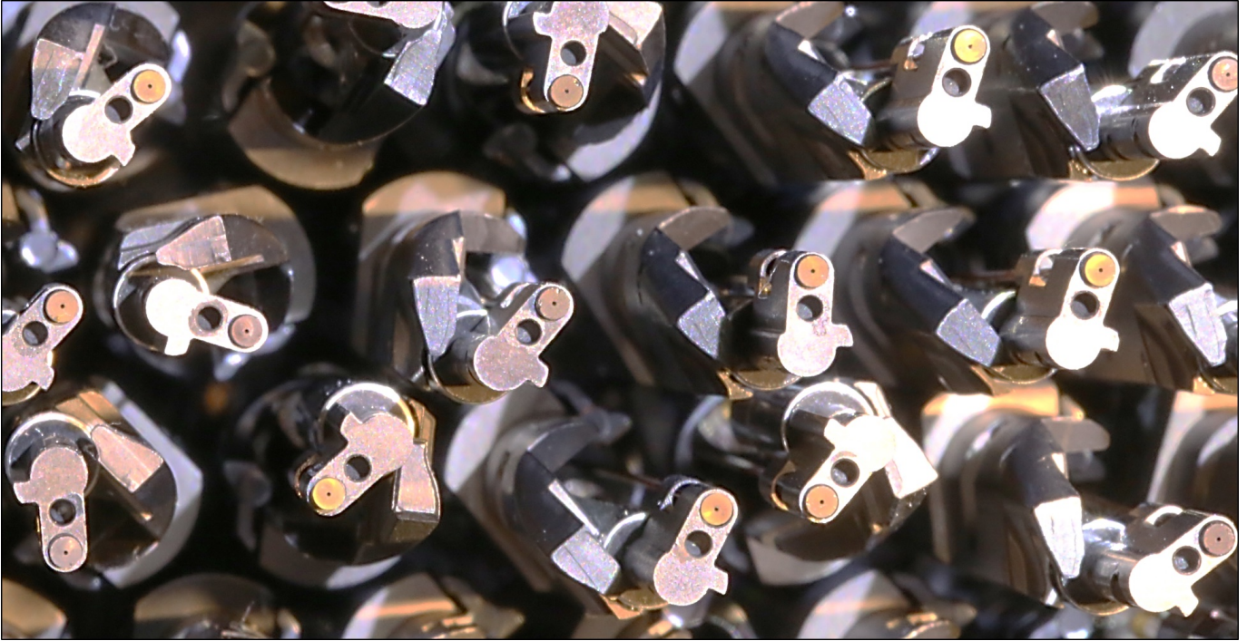
Figure 5. Fiber positioner robots are shown packed together on the focal plate. In addition to the fiber ferrule, each \phi arm has a light-trap hole with a dark dye. The original concept for these light-traps was to be able to selectively extinguish bright stars in the field; in practice they have been most useful for identifying \phi angles during hardware debugging. A projecting tab feature on each ferrule holder provides a simple but effective hard limit against clockwise over-extension.
