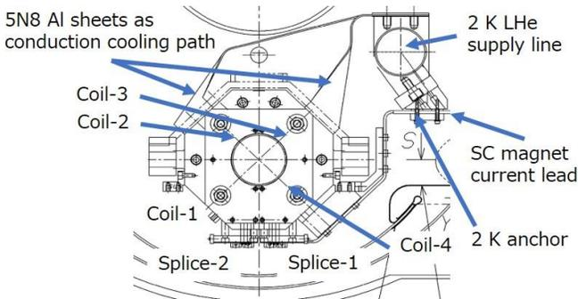
Fig. 2. Cross section drawing of installed SCQ magnet.
