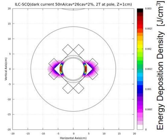
Fig. 8. Numerical simulation result of energy deposition density at the SCQ.
