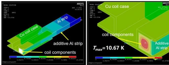
Fig. 11. Numerical simulation results with an additive aluminum strip.
