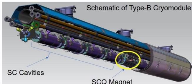
Fig. 1. Schematic of Type-B cryomodule of ILC. The Type-B cryomodule consists of 8 superconducting RF cavities, and a superconducting magnet package.
