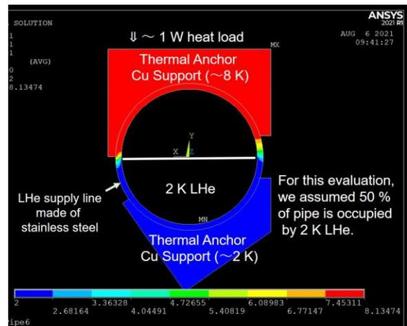
Fig. 4. Numerical calculation results of thermal profile confirmation.
