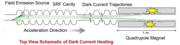
Fig. 7. Schematic of field emissions from cavity and heating at SCQ.
