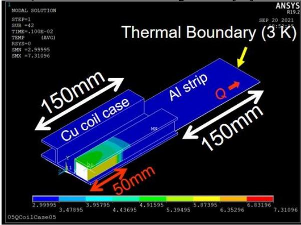
Fig. 9. FEM simulation setups to investigate thermal profiles of model coil.
