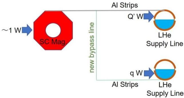
Fig. 5. Improved thermal pass with a new bypass line.
