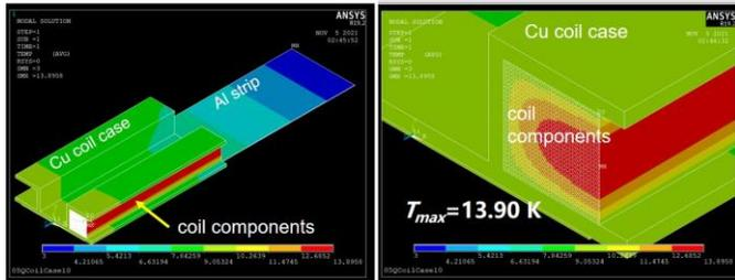
Fig. 10. Numerical simulation results of steady state with dark current heating.
