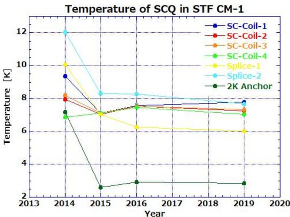
Fig. 3. Installed SCQ temperature transition plot.
