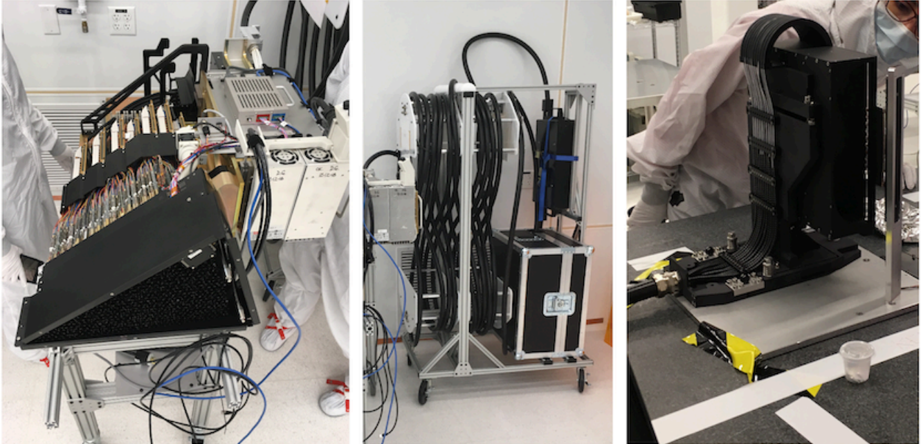
Figure 9. Photo of one of the ten DESI petal assemblies on 21 February 2019 in a cleanroom at the LBNL. The petal assembly includes the petal, fiber cable, and slithead. ( Left ) Petal with all 502 positioners, 12 fiducials, and the GFA unit, which will be aligned with the focal surface produced by the corrector. The black, triangular structure is a temporary, protective housing around these components. Behind this structure are the FIPOS electronics that drive the fiber positioners and fiducial LEDs, and wire and fiber guides. The petalbox electronics are to the right. ( Middle ) The \sim 50 m fiber cable that will extend from the petal in the focal plane system to a slithead in one of the ten spectrographs. In this photo the slithead is inside the protective case on the lower right on the cart. ( Right ) One of the DESI slitheads. The fiber cable attaches from the left in this photo. The pseudo slit of fibers is pointed at an illumination system on the right.
