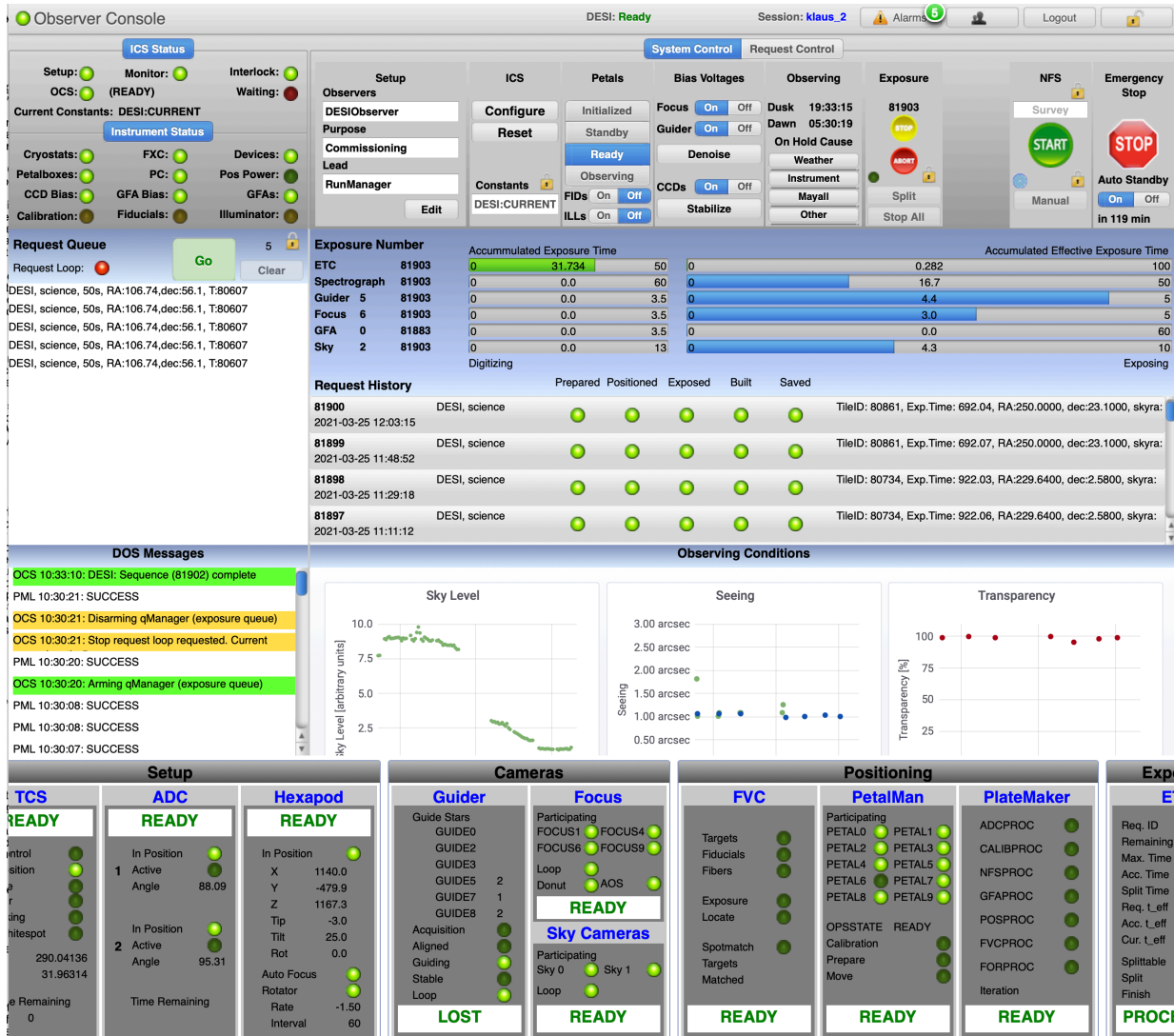
Figure 19. Screenshot of the DESI Observer Console running in a web browser window. The top section provides status information (ICS Status and Instrument Status) and elements to control the instrument (System Control and Request Control). The center section shows the observing queue (Request Queue), the ongoing exposure (Exposure Number), and the exposure history (Request History). This is followed by information on the observing conditions (Sky Level, Seeing, Transparency). The bottom section provides more detailed status information on key components of the instrument (e.g., Cameras, Positioning). Additional GUIs not shown here provide more detailed information about the instrument status and ongoing information about the most recent observation.
