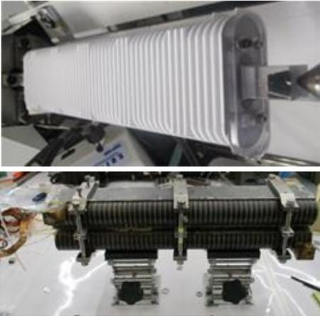
Fig. 1. Photographs of the undulator magnets after the  $\text{Al}_2\text{O}_3$  plasma spray layer (top), and assembly in the undulator configuration (bottom).
