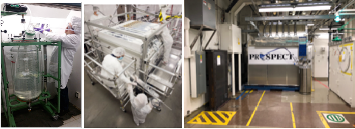
FIG. 17: Ton-scale fabrication and deployment of metal-doped liquid scintillator for Prospect
