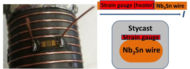
Fig. 2. Strain gauge used as heater mounted on wire (left) and experiment schematic, showing the strain gauge mounted on a flat-rolled wire (right).
