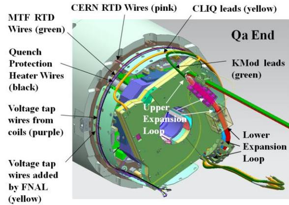
Fig. 8. Qa end of cold mass, showing bus, expansion loops and instrumentation wires.
