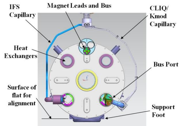
Fig. 12. Model of end view of cold mass showing support foot and capillaries.
