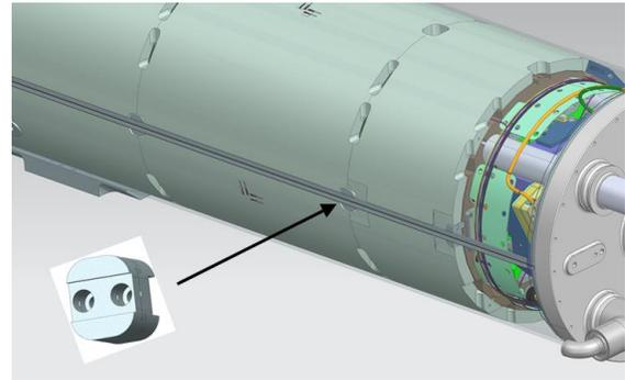
Fig. 5. Tack block position connecting magnet and cold mass. Tack blocks are placed at all interfaces between sections of the magnet outer aluminum tube. This illustration shows the tack block and backing strip installed on the magnet before the cold mass shell is added.
