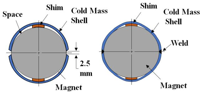
Fig. 6. Shell aligned on magnet before welding (left) and after welding (right). The space shown before welding is exaggerated for illustration. Typical shim thickness is approximately 1mm, with the space between shell and magnet outside diameter not larger than about 1mm thick before welding.
