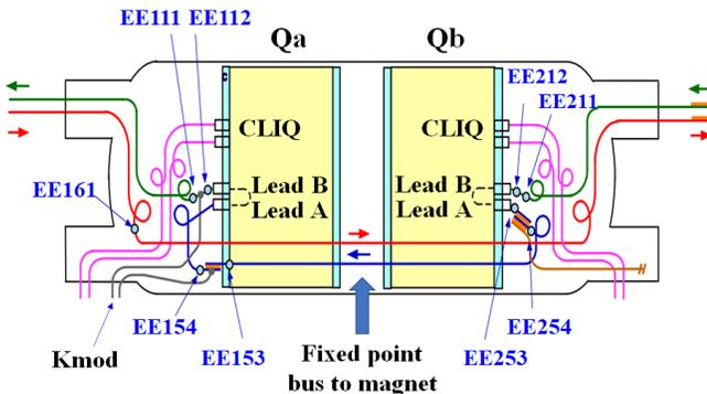
Fig. 7. Schematic of bus system. “B” lead is shown in green, “A” lead and local bus are shown in blue, through bus is shown in red, CLIQ leads are shown in pink, and Kmod leads are shown in grey. “EE” labels represent voltage taps added during cold mass assembly.
