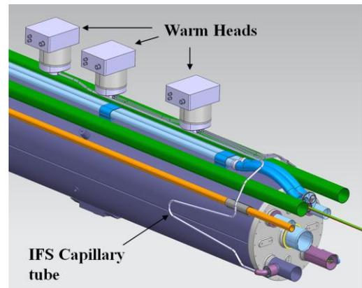
Fig. 11. Routing path of instrumentation wires. Wires are routed through the IFS Capillary and terminated to connectors at the warm head. CLIQ and Kmod wires are routed through separate capillaries on the other side of the cold mass to separate warm heads.
