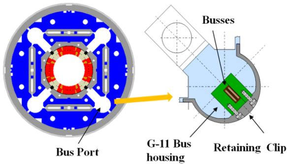
Fig. 10. Cross section of bus assembly shown as installed at right, with the bus port within the magnet shown at left.
