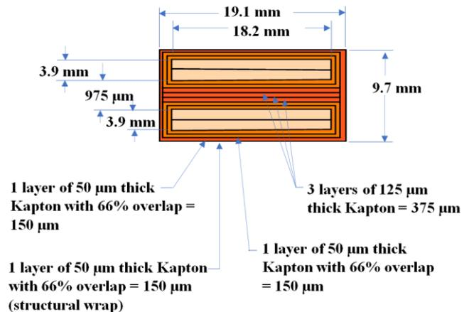
Fig. 9. Cross section of bus with insulation. The through bus is on top with the local bus beneath. The “structural wrap”, which surrounds both busses, described in the text, is used to withstand the opposing forces of the through bus and the local bus.
