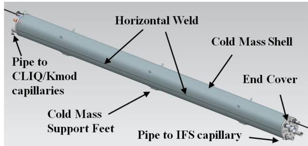
Fig. 3. Completed cold mass with stainless steel shell
