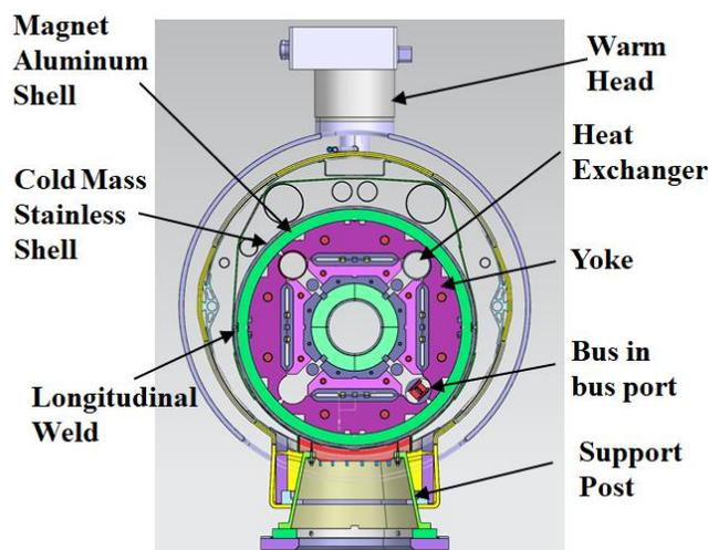
Fig. 1. Completed Cryo-assembly
