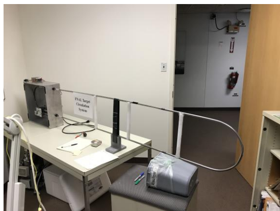
Figure 5. The first prototype of the conveyor target. (Left): as constructed. (Right): a CAD model used in the fabrication.
