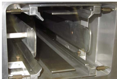
Figure 1: Photograph of one ESQ station. The top and bottom plates are held at positive voltages and the lateral plates are held at negative voltages for the vertical confinement of positive muons. The vertical magnetic field in the storage ring largely contributes to stable motion in the horizontal direction, in spite of the defocusing radial gradient from the ESQ inner and outer plates.
