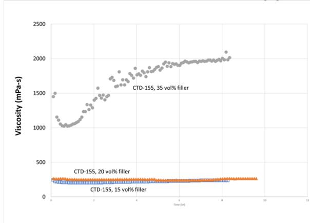
**Figure 1.** Pot life at 60°C for CTD-155 with various levels of nano-alumina filler.
