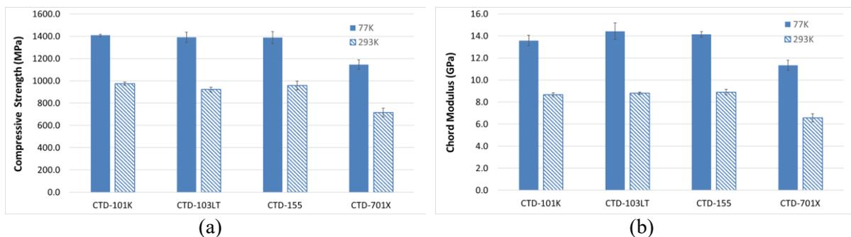
**Figure 8.** Compressive properties of S2 glass-reinforced laminates fabricated with high strain resin candidates (a) compressive strength and (b) chord modulus. Data for CTD-101K laminates are included for comparison.
