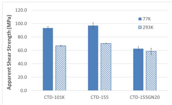
**Figure 3.** Comparison of shear performance of S2 glass laminates using CTD-155 resin variants. Data for CTD-101K laminates is included for comparison.
