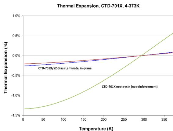
**Figure 11.** Thermal expansion of CTD-701X with and without reinforcement.
