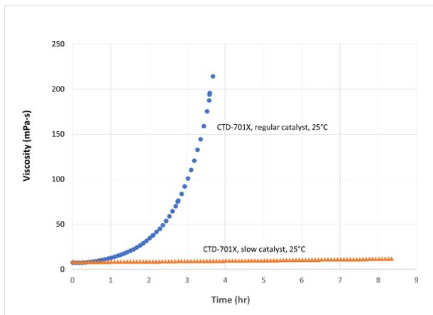
**Figure 7.** Pot life of CTD-701X at 25°C with two different catalyst systems.
