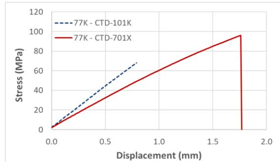
**Figure 6.** Neat resin stress-deflection curves at 77 K for CTD-101K and CTD-701X
