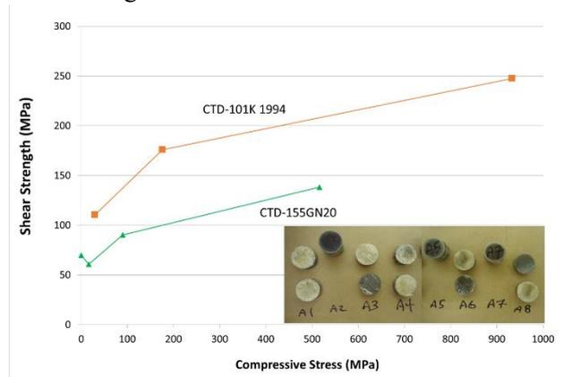
**Figure 4.** Shear compression test results for S2 glass/CTD-155GN as compared to results for S2 glass/CTD-101K. Inset photograph shows failure surfaces in the test specimens.
