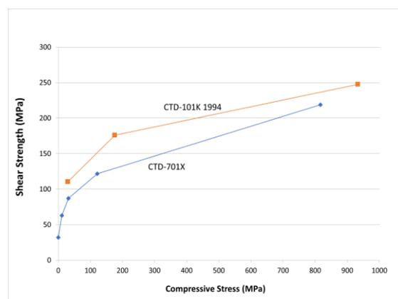
**Figure 10.** Shear compression test results for S2 glass/CTD-701X as compared to results for S2 glass/CTD-101K.
