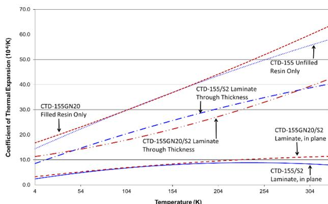
**Figure 5.** Comparison of thermal expansion for CTD-155 and CTD-155GN20 laminates and unreinforced resins.
