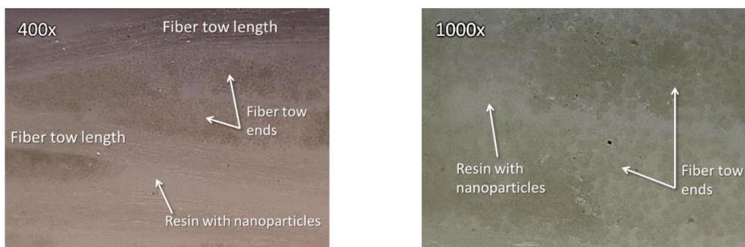
**Figure 2.** Optical microscopy of S2 glass/CTD-155GN laminate. Notice the uniformity of the laminate; no particle separation visible, resin area is a uniform milky white color with no “clear” spots or voids.
