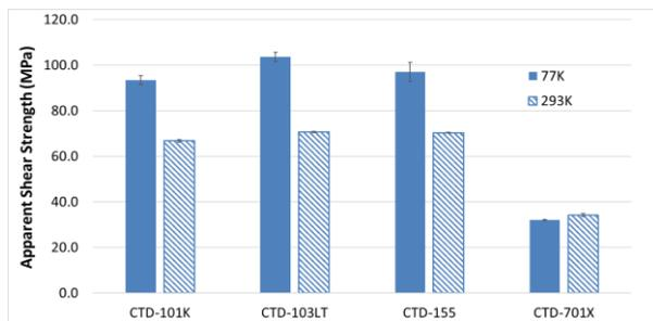
**Figure 9.** Apparent shear strength of S2 glass-reinforced laminates fabricated with high strain resin candidates. Data for CTD-101K laminates are included for comparison.
