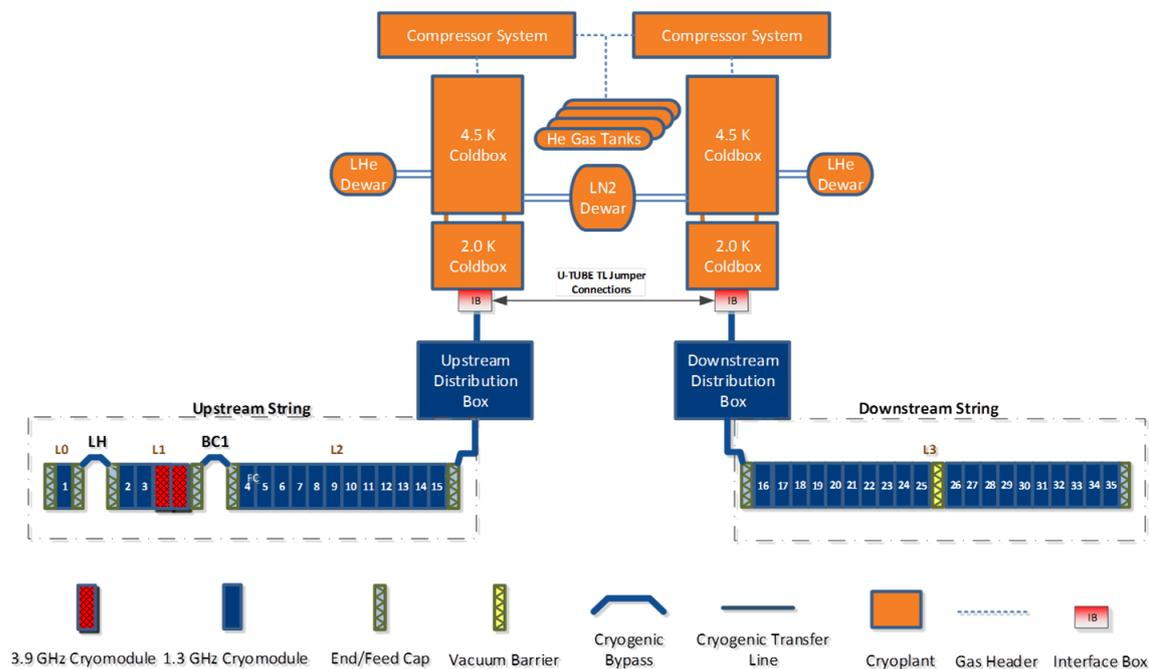
**Figure 1.** LCLS-II cryogenic system overview.
