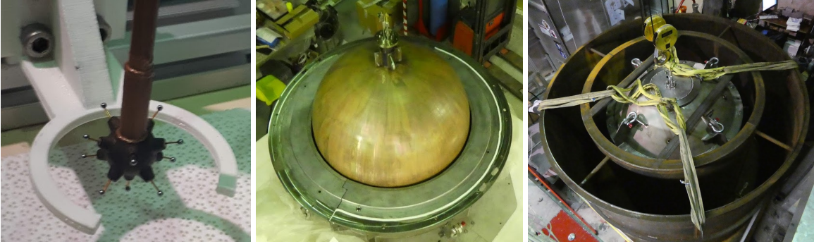
Figure 19: NEWS-G’s S140 setup at LSM (2019). From left to right: ACHINOS anode; S140 sitting on the lower half of the lead shield; S140 in the closed lead shield, inside the open water shield.
