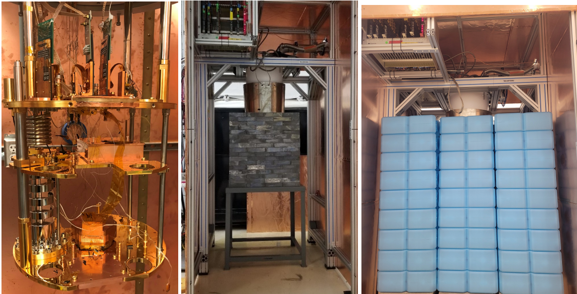
Figure 5: (left) Typical detector mounting inside the MINER Bluefors fridge, similar to how SuperCDMS test facilities mount the detectors. The SQUIDs are mounted at the 600 mK stage. The detector stack is designed to provide 1-inch internal hermetic shielding surrounding the detectors to reduce radioactive background, (center) 4-inch lead shielding surrounds the fridge with an open top, (right) 55% borated rubber sheets of 2mm thickness surround the lead shielding to capture thermal neutrons. Water bricks of 8-inch thickness surround the entire setup except for the open top. External neutrons are moderated by the water shielding and then captured efficiently by the borated rubber shielding, with the lead shielding providing shielding against external gammas and the gammas from the thermal neutron capture in boron.
