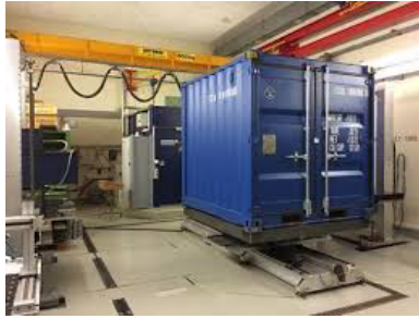
Figure 3.15: Movable support structure for concept evaluation. Its movement degrees of freedom allow 3D \gamma -ray beam scanning for “real-world” scenarios. This figure is adapted from a paper by Kolokytha et al. [136] of the CEA Saclay in France.
