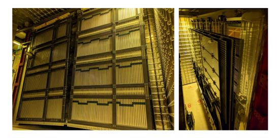
**Figure 76**: . Left: Salève-side drift FC end-walls are ready to be deployed inside the cryostat. Right: CPA and FC assemblies inside the cryostat ready to be pushed to their final position.
