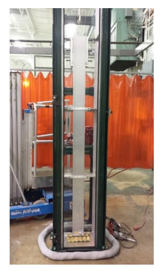
Figure 40: Mechanized dipping setup at Fermilab, used for the production of dip-coated light guides.
