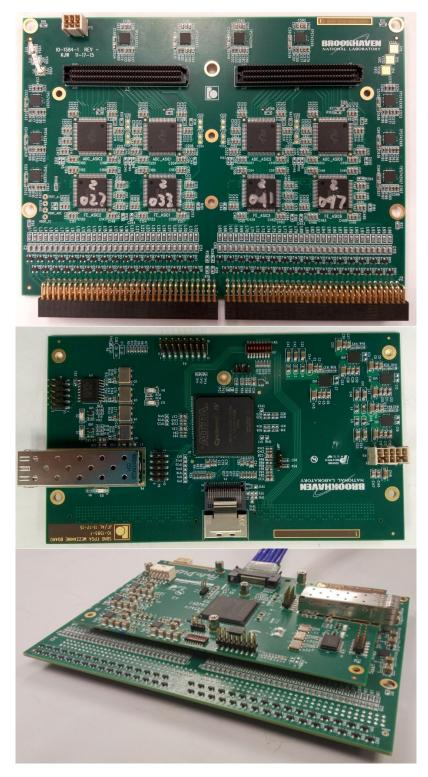
**Figure 33**: The Front End Mother Board (FEMB). Top: The analogue mother board, showing four ADC ASICs and four FE ASICs, surface mounted. The other side of the board has another four ADC and FE ASICs. Middle: The FPGA mezzanine. Bottom: The complete FEMB assembly. The cable shown is the high-speed data, clock, and control cable.
