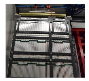
**Figure 20**: Endwall FC assembly, the stacked modules are visible. The endwall is hung in front of the cryostat before insertion through the TCO. The visible face is the one that will face the inside of the detector active volume. The dark grey FRP plates are the support structure of the endwall and interconnected between the volumes.
