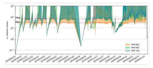
**Figure 57**: The electron lifetimes measured by three purity monitors in ProtoDUNE-SP as a function of time, September 2018 through February 2020. The purity is low prior to the start of circulation in October 2018. Later dips represent recirculation studies and recirculation pump stoppages. The shaded bands represent uncertainties of the measurements.
