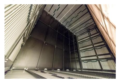
**Figure 14**: One of the two drift volumes of ProtoDUNE-SP. The FC modules enclose the drift volume between the CPA array (at the centre of the image) and the APA (upper right). The endwall FCs are oriented vertically; the top and bottom units are horizontal. The staggered printed circuit boards connecting the endwall FC profiles are the voltage divider boards.
