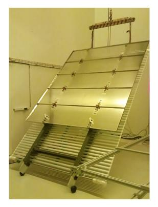
**Figure 18**: Lifting of a Top FC module for subsequent installation on the CPA panel. The side of the FC module that is lifted will attach to the CPA while the other side (bottom side) is connected with latches to the APA.
