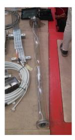
**Figure 66**: A photo of the ProtoDUNE-SP warm inspection camera acrylic tube immediately before installation; the acrylic tube is sealed with an acrylic dome at the bottom and can be opened at the top.
