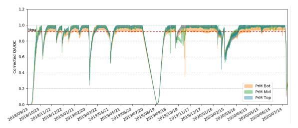
**Figure 56**: The anode-to-cathode signal ratios measured by three purity monitors in ProtoDUNE-SP as a function of time, September 2018 through February 2020. The purity is low prior to the start of circulation in October 2018. Later dips represent recirculation studies and recirculation pump stops. The shaded bands represent uncertainties of the measurements.
