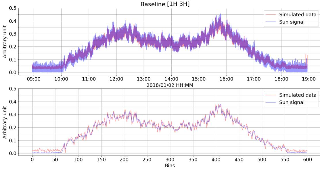
**Figure 23.** Top: The difference between the simulated visibility (shown in Fig. 20) and Sun-removed visibility (shown in Fig. 21) is shown in red. The signal from the largest eigenvector, which is used as the Sun signal during the daytime is shown in blue. Bottom: Same plot over the same time interval but the data are averaged in 60 second time bins to reduce the noise.
