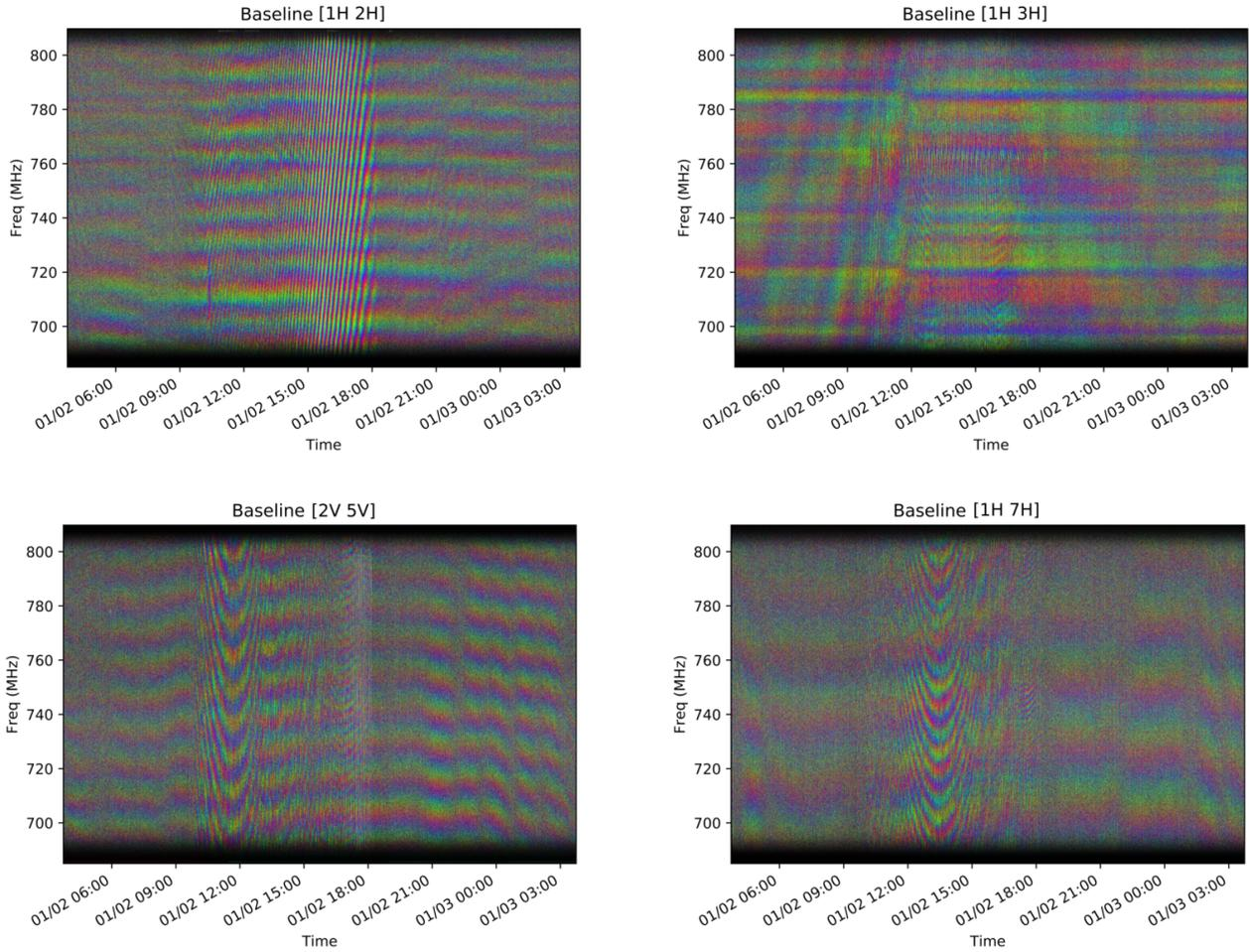
**Figure 15.** The waterfall plot of the complex visibility after zeroing the largest eigenvalue during daytime for four typical baselines. Nightly mean subtraction has been applied. There is still some residual solar contamination signal, which is causing the weak fringes during the daytime.
