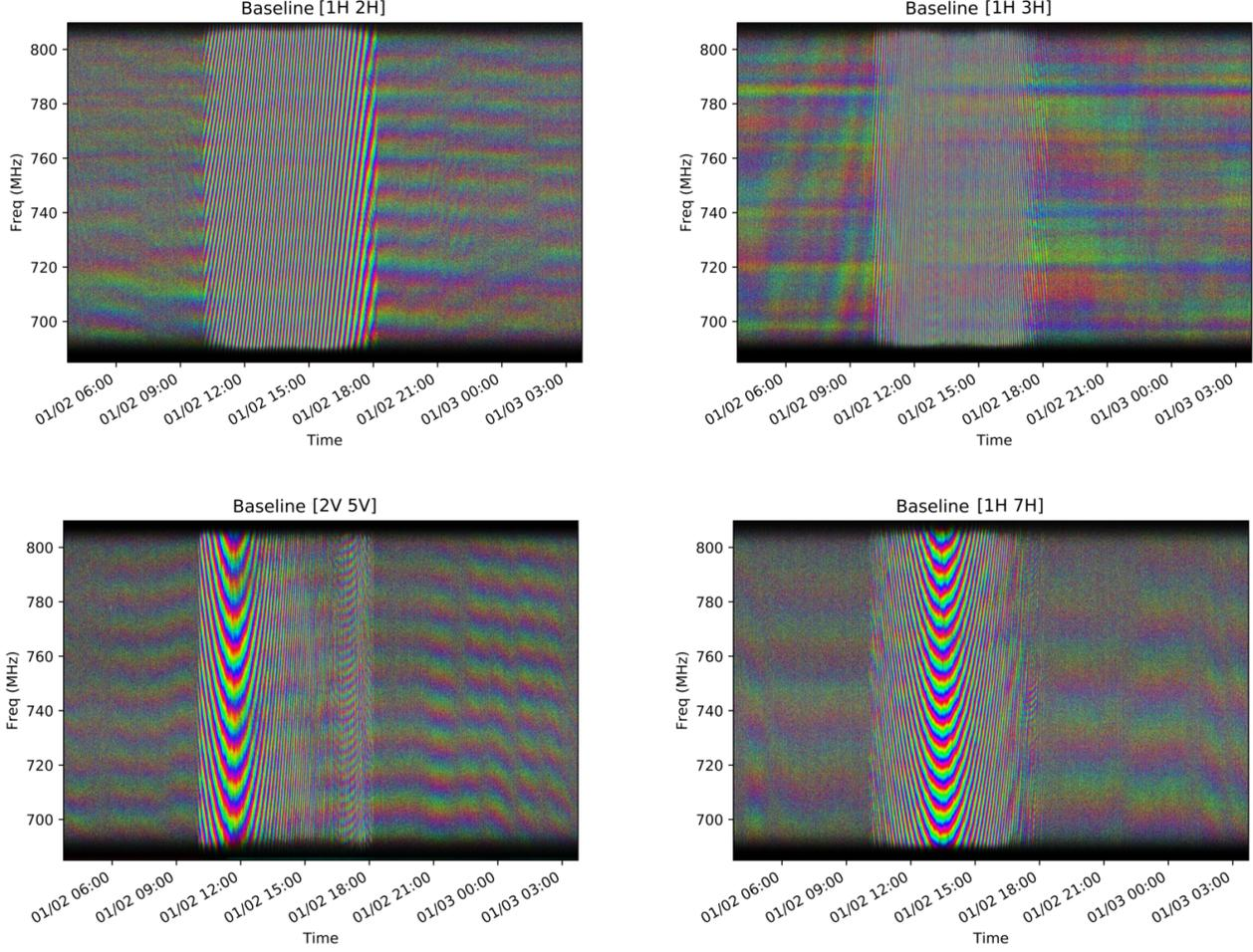
**Figure 9.** The waterfall plot of the complex visibility (same as Fig. 7) after the nightly mean subtraction. We can see that most of the horizontal stripes, which probably are caused by cross talk, are now gone from the waterfall plot. The structures from the sky are more prominently visible.
