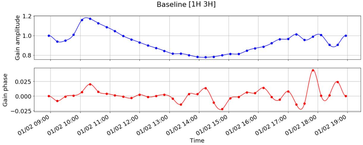
**Figure 18.** Plot of the gain  $g = Ae^{i\phi}$  after  $\chi^2$  minimization for 10 hours during the daytime. Blue: Plot of the gain amplitude  $A$ . Red: Plot of the gain phase  $\phi$  in radians. The dots represent the points of  $\chi^2$  minimization that occur every 1000 seconds. These gain values are extrapolated to the intervening points for a total of 36,000 seconds.
