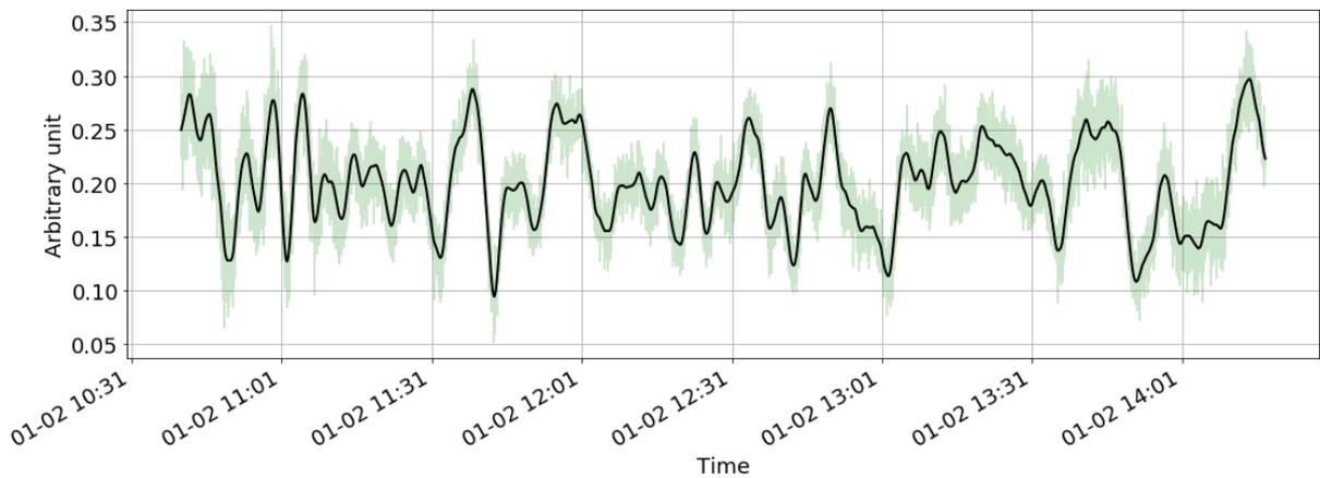
**Figure 16.** A 4-hour segment of the amplitude of one component of the eigenvector corresponding to the largest eigenvalue is shown in the light green curve. The sampling interval is 1 s. The random fluctuations in the data come from the noise. The black curve shows this component after smoothing the data, as described in section 4.1.
