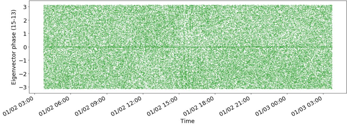
**Figure 12.** Phase plot of the 15th component of the eigenvector corresponding to the 4th largest eigenvalue in the horizontal polarization visibility  $\mathbf{V}^{(H)}$ . Here we don't see any fringes, showing that no individual strong source is contributing to this particular eigenvalue.
