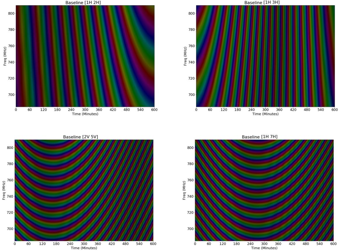
**Figure B1.** Combined visibilities of three artificial sources for different baselines, shown here for 10 hours. As expected, longer baselines give higher fringe rates, and for a given baseline, we see a faster fringe rate at lower frequency.
