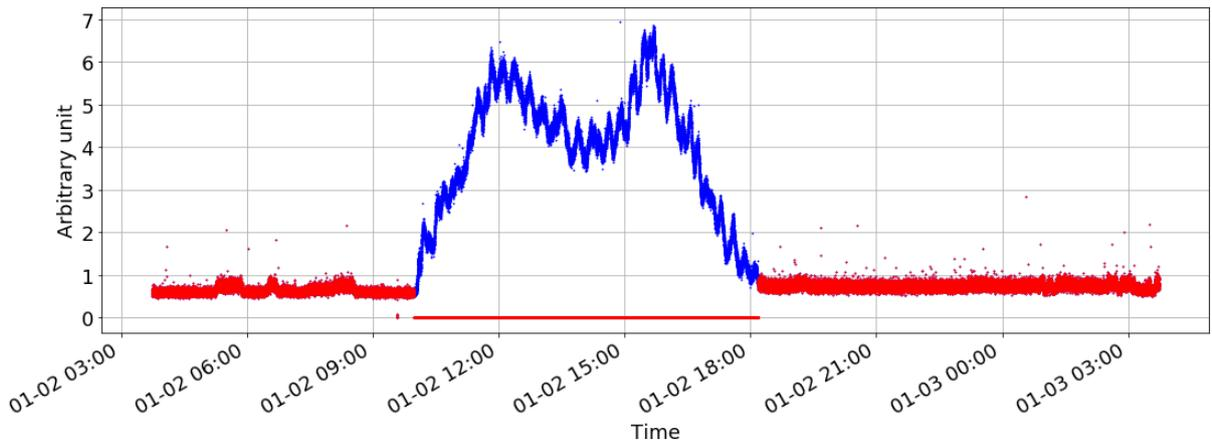
**Figure 14.** Blue: The original largest eigenvalue from the eigen-decomposition, during daytime. Red: The same largest eigenvalue but with zero value during the daytime. This step simulates removing the Sun signal in Eq. 11, since the largest eigenvector during the daytime points in the direction of the Sun in the eigenspace.
