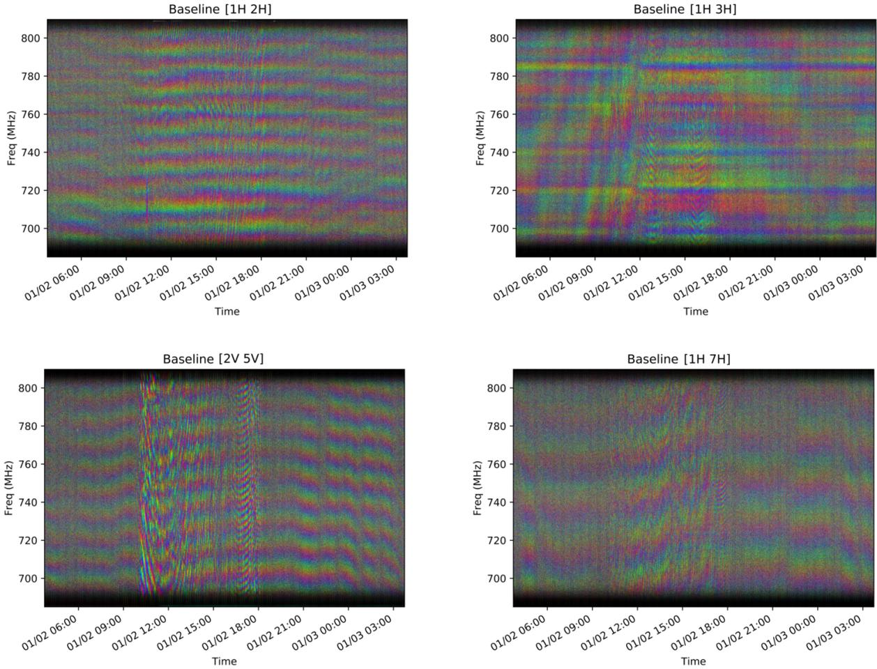
**Figure 19.** The waterfall plot of the complex visibility after  $\chi^2$ -optimization scaling the Sun signal by a gain factor (Section 4.2) for four typical baselines. We can see that most of the sun signal contribution has been removed. However, very weak noisy fringes are still visible during daytime, specially in some baselines, such as in [2V 5V], shown in the bottom left panel.
