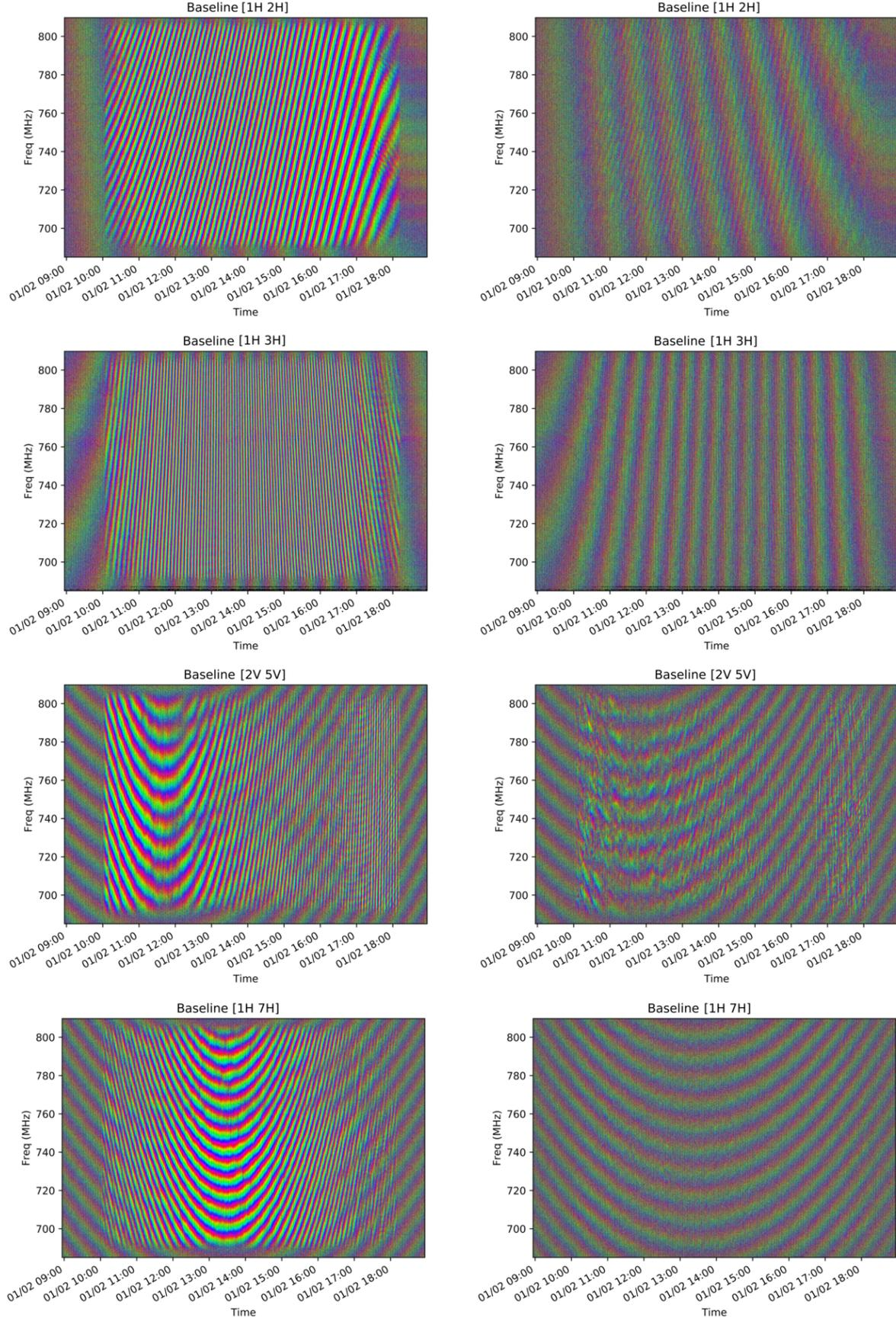
**Figure 24.** Left column: Simulated daytime visibilities for several baselines. The bright fringes are from the Sun and the weaker fringes are from the artificial sources. Right column: Sun-removed visibility using AlgoSCR. The fringes from the artificial sources are clearly visible. We can see that most of the solar contamination is removed by AlgoSCR.
