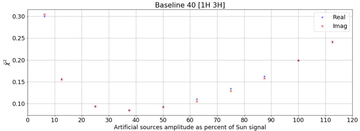
**Figure 26.** Plots of  $\bar{\chi}^2 = \frac{1}{n_t |V_{\text{org}}|} \sum_{t,\nu} (V_{\text{org}} - V_{\text{sim}})^2$  from the real and imaginary parts of the visibility for different artificial source amplitudes. Here, the plots are normalized by  $|V_{\text{org}}|$  instead of  $\sigma^2$ . We can see that the  $\bar{\chi}^2$  is lowest at about 40, indicating that the recovery is best when the amplitude of the source is about 40% of the Sun signal.
