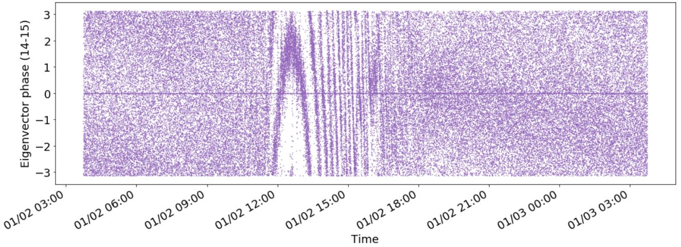
**Figure 13.** The phase of one component of the eigenvector corresponding to the 2nd largest eigenvalue. We can see weak fringes, indicating that some of the solar contribution is present in the second largest eigenvalue.
