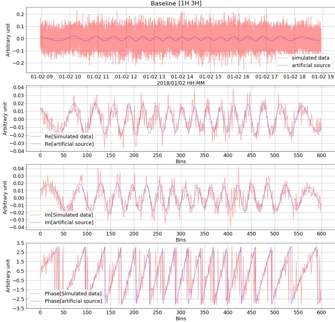
**Figure 21.** Top: the real part of the Sun-removed visibility from simulated data for baseline [1H 3H]. The signal from the artificial sources is shown in blue. The visibilities are sampled every second. The lower three plots show the real part, imaginary part, and phase of the Sun-removed visibility, after 60-second averaging.
