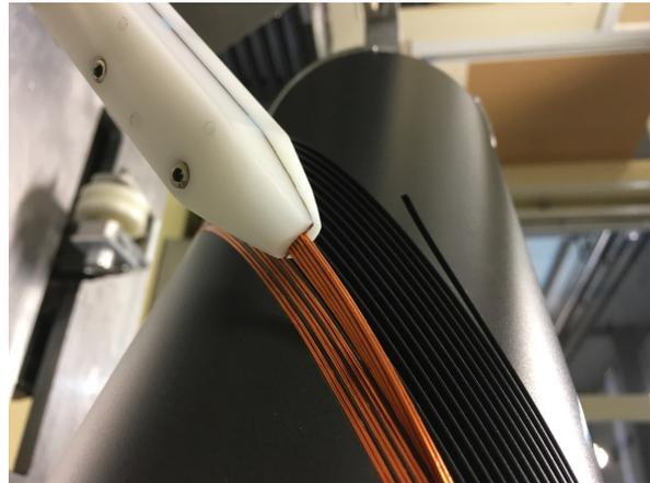
Fig. 7.87: Tooling allowing to wind ten strands in one go.
