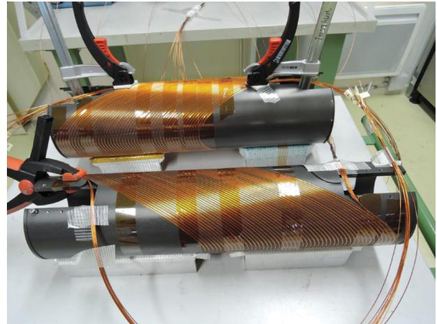
Fig. 7.1: Two tilted solenoids of the short model of the canted corrector before being inserted one into the other.
