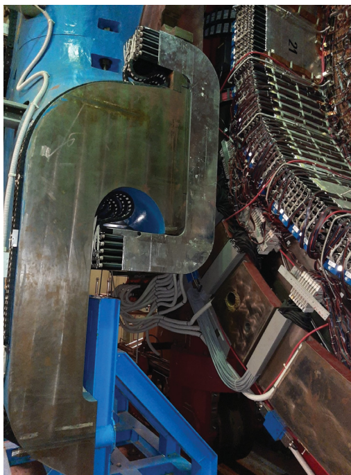
Figure 5.3: (left) A part of the KLOE magnet near one of the end caps. (right) The magnitude of the longitudinal (i.e., along the magnet symmetry axis) component of the magnetic field (in Gauss) as a function of the position along the magnet axis (in cm), measured from the center ( z = 0 cm) toward the end cap ( z \approx 200 cm). Data and MC are compared. The field was measured and simulated on the magnet symmetry axis.
