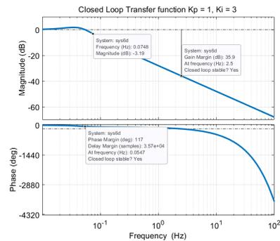
Figure 5: Closed Loop Frequency Response for  $K_I = 3, K_P = 1$ .
