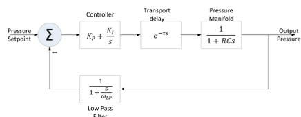
Figure 4: Tuner Control System Model.
