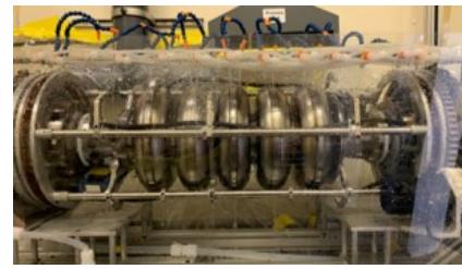
Figure 2: Bulk electropolishing of B61-EZ-001 at ANL EP facility [9].
