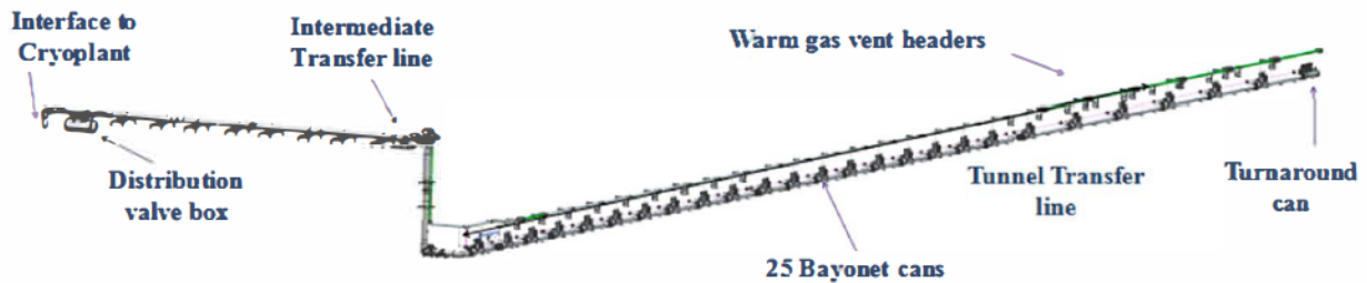
Figure 1. Schematic of the PIP-II Cryogenic Distribution System.
