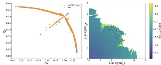
Figure 2: Left: Tune footprint of the IOTA lattice with octupoles, obtained with pyORBIT and MADX. Right: Difference in tune shifts (on a log scale) between pyORBIT and MADX as functions of the initial positions of the test particles.
