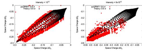
Figure 6: Tune shifts with amplitude due to space charge from pyORBIT and theory at intensity  $10^{10}$  (left) intensity  $9 \times 10^{10}$  (right).
