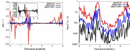
Figure 5: Symplecticity tests with space charge.  $\det J - 1$  (left) and  $\|J^T S J - S\|$  (right) as functions of the transverse amplitude in units of the rms beam size.
