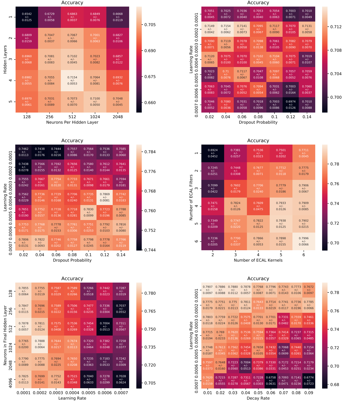
Fig. 11. Selected hyperparameter scan results for DNN (top), CNN (center), and GN (bottom). In each figure, the classification accuracy is displayed as a function of the hyperparameters reported on the two axes.
