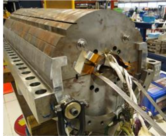
280 Figure 10. Bi2212 and 60-mm aperture 2-layer Nb 3 Sn half-coils inside HFDM dipole mirror structure (left); and 281 a picture of the HFDM mirror structure with 60-mm Nb 3 Sn coil inside (right) [16]. 282
