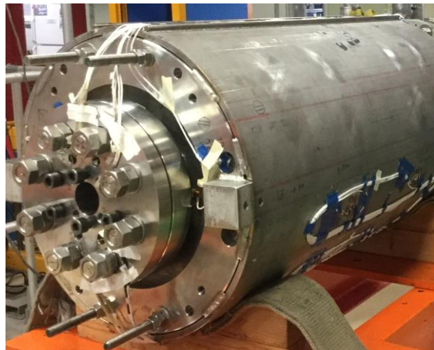
284 Figure 11. Cross-section of 6-layer hybrid dipole coil inside MDPCT dipole structure (left); and a picture of the 285 MDPCT1 dipole with 4-layer Nb 3 Sn coil inside (right) [18]. 286
