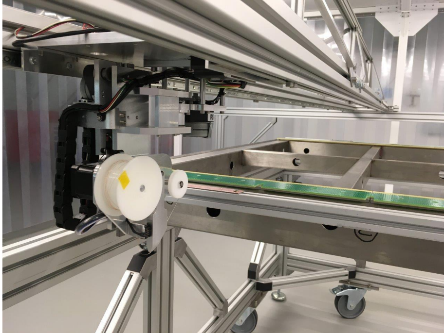
Figure 25. The wiring head, ready to start wiring trials.
