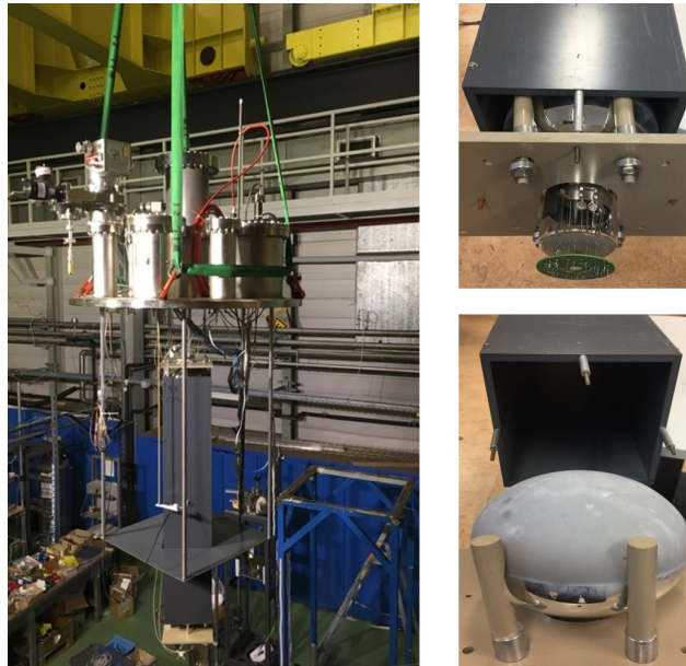
Figure 3: Left: Experimental setup during the insertion in the liquid argon cryostat. Right: Picture of one internal PMT on its PEEK support (bottom) and in the final position inside the box (top).
