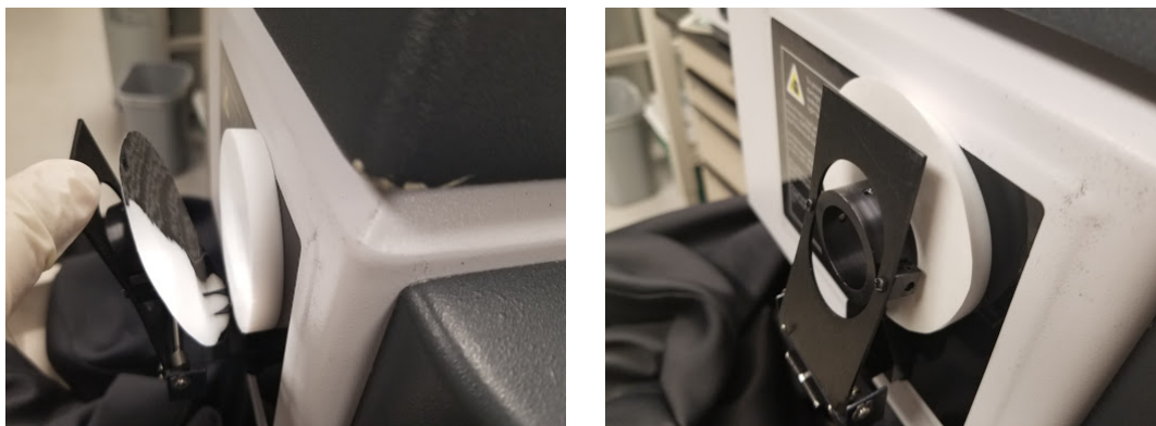
Figure 7: Left: 3M foil being installed at the back of a disk of PTFE at the mouth of the integrating sphere. Right: 3M foil held on the back of a PTFE disk by the SPM lever arm.
