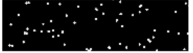
FIG. 4. Section of a Skipper-CCD image after exposing it to the X-rays emitted by the ^{55}\text{Fe} radioactive source where different cluster size can be identified.
