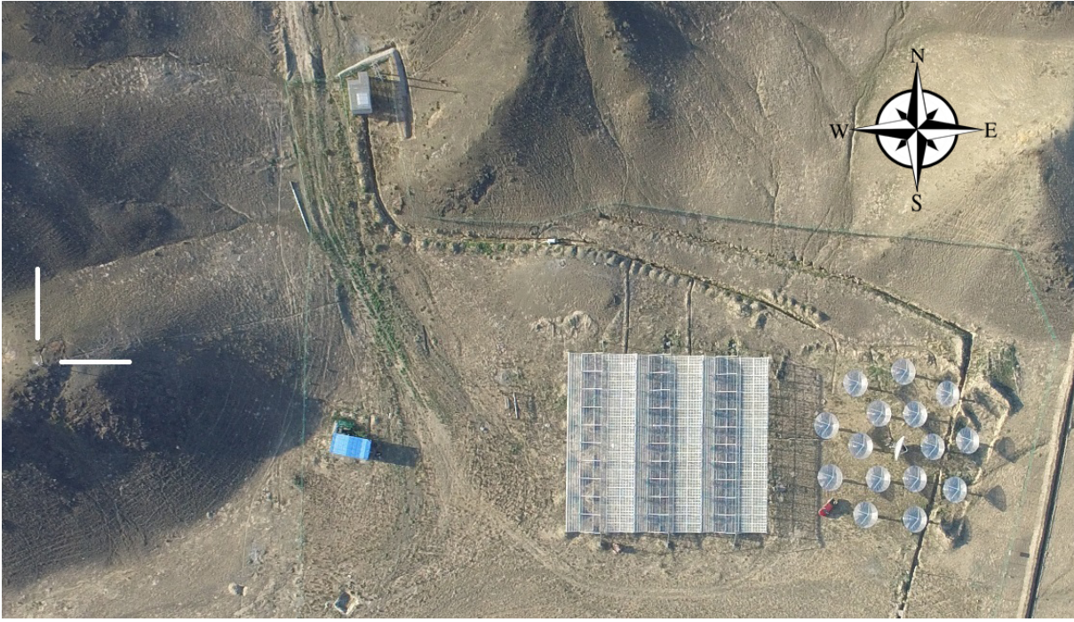
Figure 1: A top view photograph of the Tianlai cylinder and dish arrays. The dish is located in the east side of the cylinder, the calibrator noise source (CNS) is located on a hill to the west of the arrays, as marked on the left side of the photograph. There is a blue cabin for storage between the array and the CNS.
