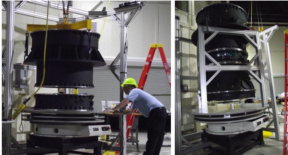
Figure 4: Left-The DESI corrector aft and middle sections being re-assembled by UCL’s Dr. David Brooks at the Mayall on the UCL precision turntable for post-shipment alignment verification. Right-The fully re-assembled corrector on the alignment turntable.
