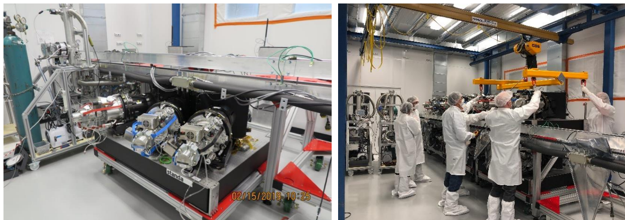
Figure 21: Left-The second installed spectrograph in the foreground, integrated with its three cryostats (shiny assemblies with red, blue, and black struts), after craning onto its lower-level rack cart. Obscured in this photograph is the first installed spectrograph, whose cryostats are being pumped down using the vacuum pump on the cart with the gas bottle on it. Right-The sixth spectrograph being lowered into its position on the top row of the rack by the shack gantry crane, using a custom spreader bar.
