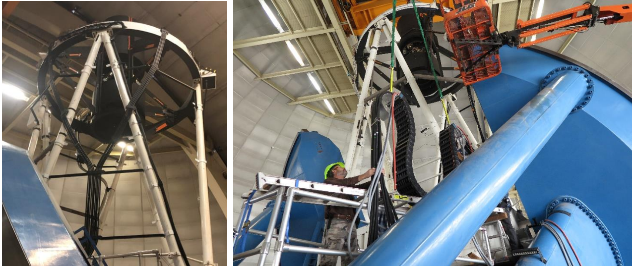
Figure 16: Left-The two groups of five fiber cables are supported by custom mounting hardware designed and built by NOIRLab, forming a 'Y' from the upper ring down toward the telescope declination axis. Right-Kitt Peak engineers prepare to integrate the populated articulated cable carrier around the declination axis, in the gap between the white telescope center section and the blue horseshoe.
