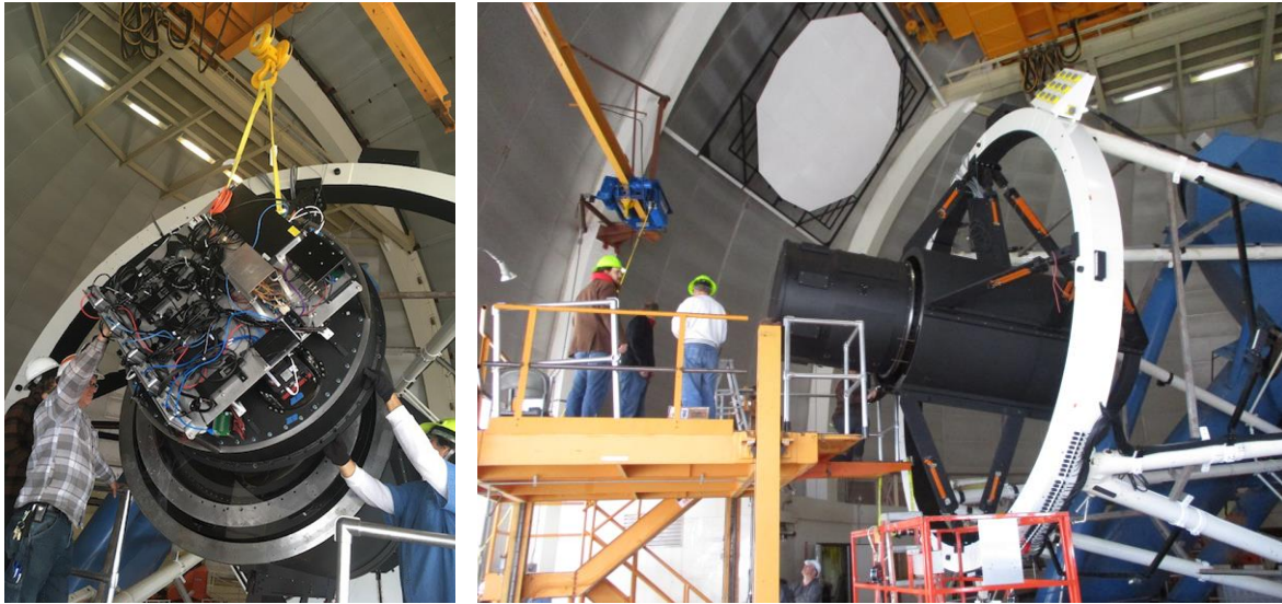
Figure 11: Left-The Commissioning Instrument focal plane assembly being positioned for installation to the DESI corrector in March 2019. Right-The Commissioning Instrument fully installed on the telescope.
