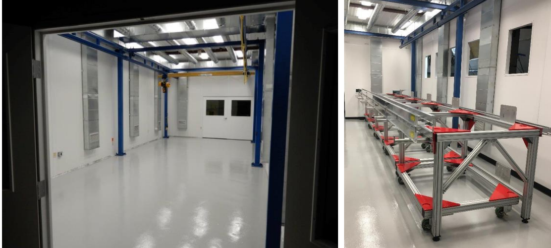
Figure 19: Left-The interior of the spectrograph clean room shack shortly after its construction and coating of the floor. The gantry crane is the yellow assembly that rides on the blue frame. Right-The spectrograph support rack in October 2018, ready for installation of the ten spectrographs in two rows of five. The upper row of spectrographs sits atop the rigid frame, while the lower row of spectrographs sit on individual carts that roll under the top row.
