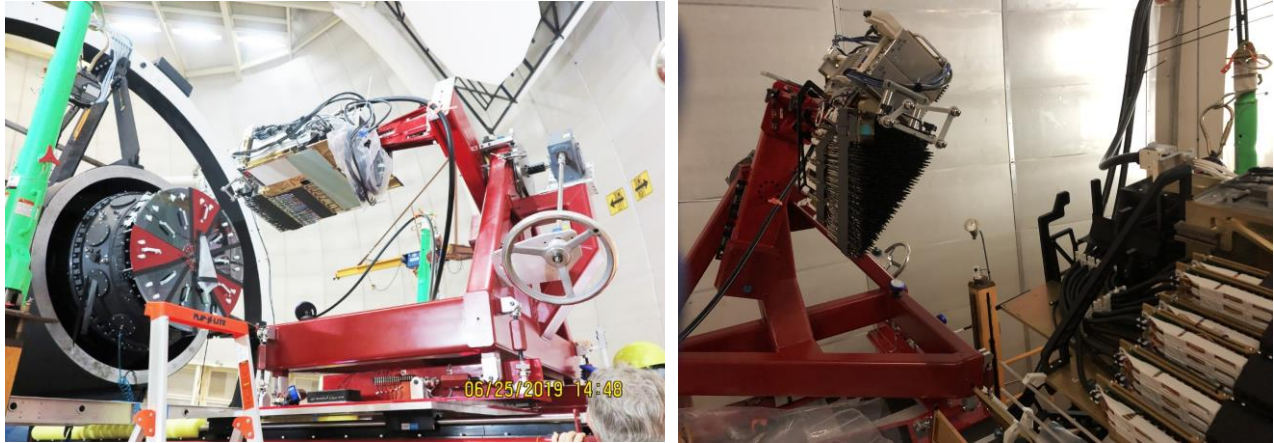
Figure 13: Left-The first of ten DESI production petals, supported on the rotary stage of the PMA, ready to be installed to the focal plane ring by advancing the Sled toward the telescope. The red and transparent wedge parts on the focal plane adapter protected the optics from the dome environment and were removed only when a petal was aligned and ready to insert. Right-A later petal ready for installation next to an already-installed petal, visible in the lower right of the photo. The bare aluminum irregular quadrilateral part above the black petal is a temporary mount for four SMRs, used to align the petal with the corrector.
