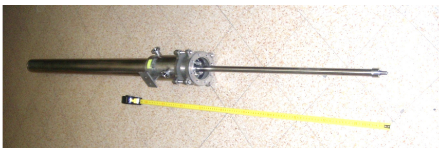
Figure 2. The adopted mechanical extendible handler.
