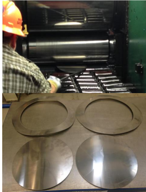
Figure 2: Rolling process at ATI (top) and final discs with cutoffs (bottom).
