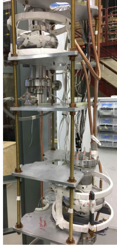
Figure 6: Large grain cavities suspended from the dewar top plate after instrumenting for expulsion measurement.
