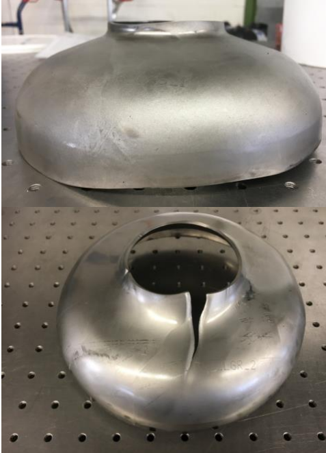
Figure 3: The non-rolled material was formed into half-cells without tearing (top), but the rolled material tore near the iris (bottom).
