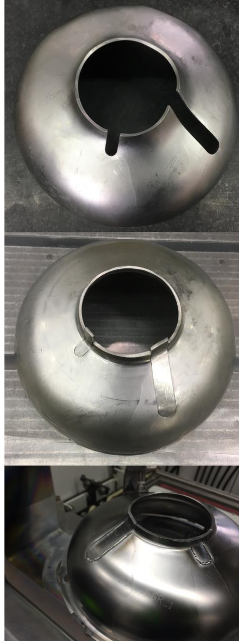
Figure 4: The repair process for the rolled half-cells involved milling out the torn section (top), inserting plugs of matching material (middle), and welding them into place (bottom).
