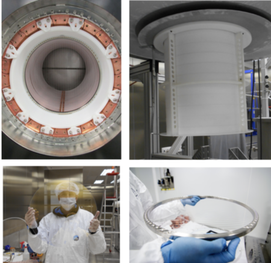
Figure 3: The main components of the TPC. Top left, the field cage, showing the HDPE body, the copper rings and the cathode grid; bottom left, the anode quartz plate; top right, the light tube; bottom right, the gate grid.
