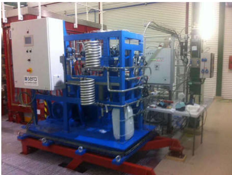
Figure 19: The NEXT-WhiteNEXT-100 compressor, manufactured by SERA.
