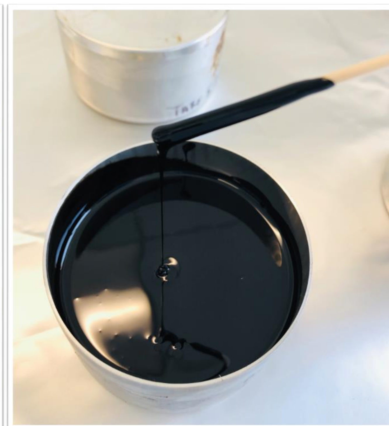
Bitumen-polymer sample prepared for electron beam treatment
