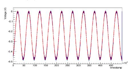
Analyzed more than 300 GB of data from neutron and TID tests, no evidence of bit flips or waveforms shape variation.
