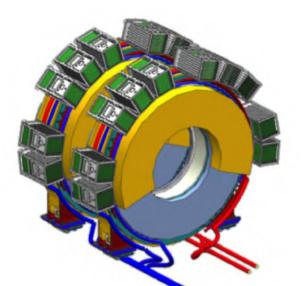
1 crystal coupled to 2 large (14x20 mm<sup>2</sup>) area UV-extended SiPM (total of 2696 electronic channels).
