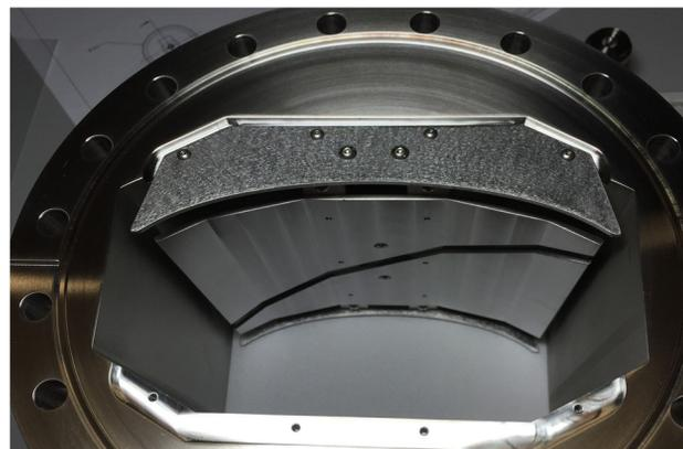
Figure 11: Elliptical beam position monitor for multi-charge state beam in Folding Segment dispersive section. The 150 mm wide horizontal aperture accommodates up to five uranium beam charge states over 80 mm spread.
