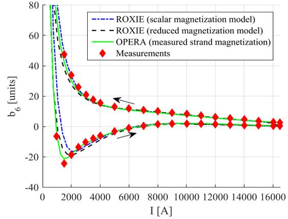
Fig. 6. Measured and calculated  $b_6$  field component as a function of the magnet current. Calculations are shifted by 0.7 units to suppress for the geometric component.
