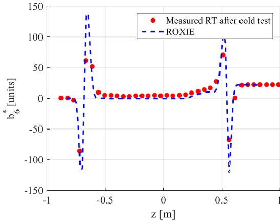
Fig. 4. Measured and calculated profile of the pseudo-harmonic  $b_6^*$  along the magnet axis measured at room temperature after cold powering test.  $z=0$  correspond to the magnetic axis of the magnet.
