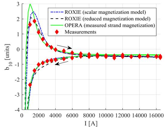
Fig. 7. Measured and calculated  $b_{10}$  field component as a function of the magnet current. Calculations are shifted by 0.1 units to suppress the geometric component
