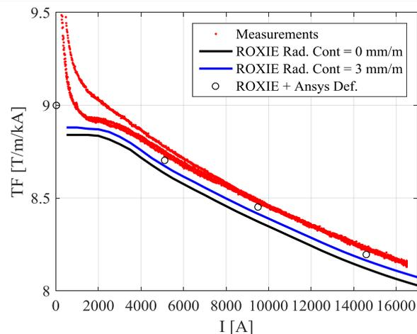
Fig. 2. Current dependence of the transfer function measured during a machine cycle to nominal current compared to ROXIE model assuming no coil deformation during cool down, a radial contraction of 3 mm/m and the coil deformation as computed with ANSYS.
