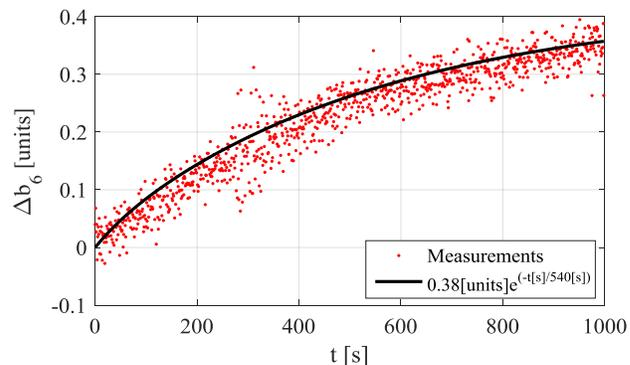
Fig. 9. Decay in the dodecapole field component at injection in MQXFS1a during the accelerator cycle. Measurements in a 100 mm length segment in the center of the magnet.
