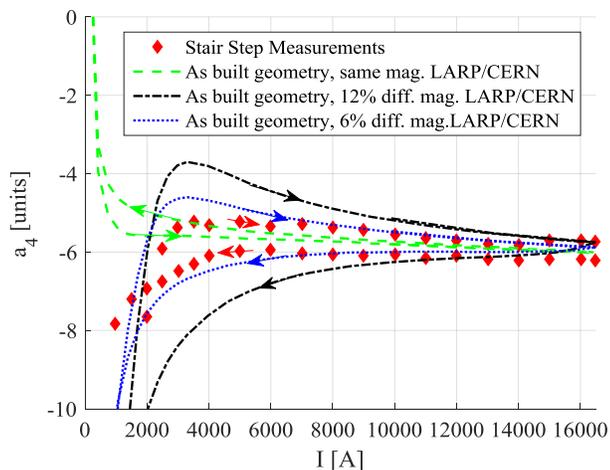
Fig. 8. Measured and calculated  $a_4$  field component as a function of the magnet current.
