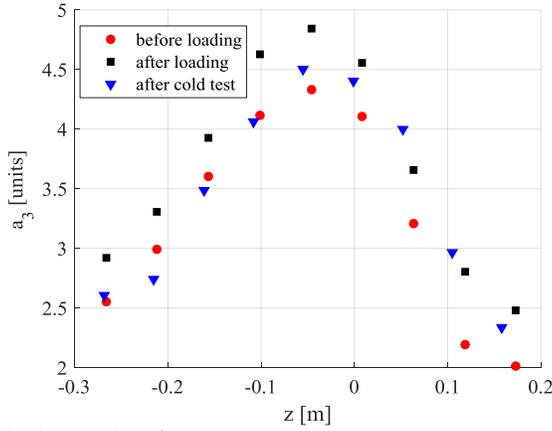
Fig. 3. Evolution of the skew normal component along the magnet axis measured at room temperature before loading, after loading and after cold test.  $z=0$  correspond to the magnetic center of the magnet.
