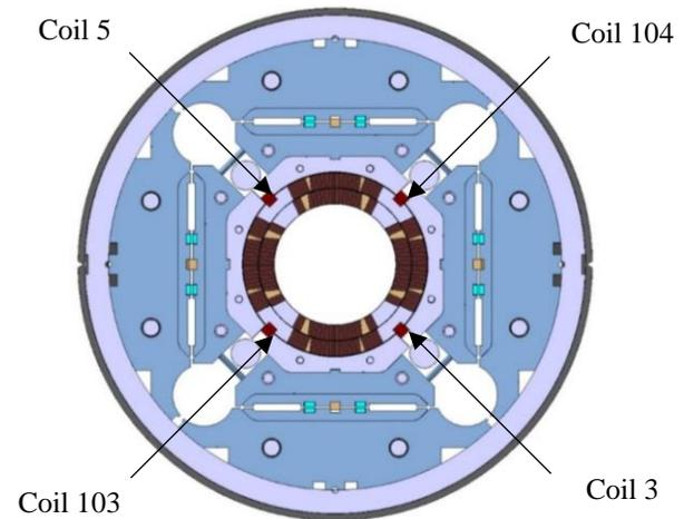
Fig. 1. Magnet cross section viewed from the lead end, including the position of each coil in the magnet assembly.
