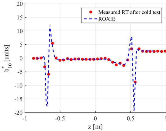
Fig. 5. Measured and calculated profile of the pseudo-harmonic  $b_{10}^*$  along the magnet axis measured at room temperature after cold powering test.  $z=0$  correspond to the magnetic axis of the magnet.
