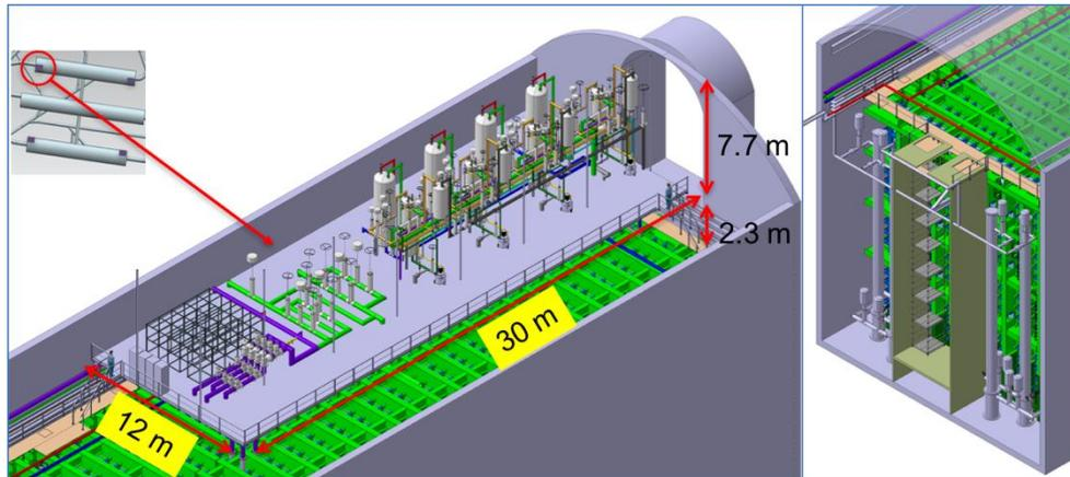
Figure 5. Proximity cryogenics in the detector cavern (mezzanine on the left and LAr pumps on the right)
