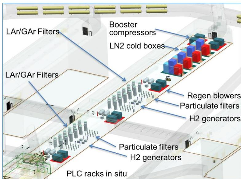
**Figure 4. Layout of the cryogenics in the Central Utility Cavern**
