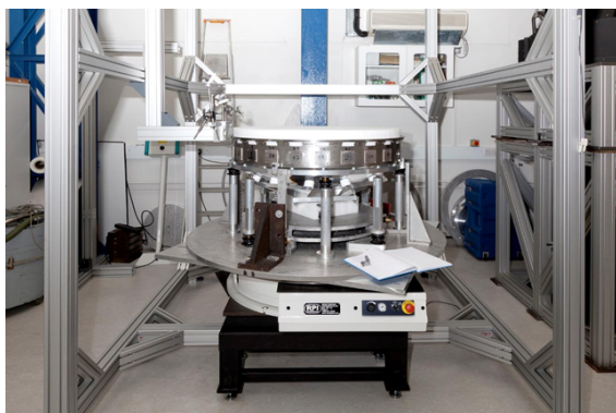
Figure 2.20: DECam C1 lens alignment setup.
