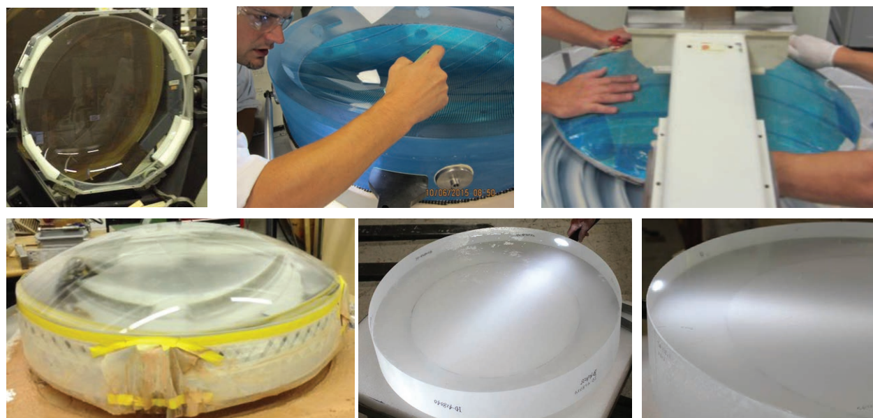
Figure 2.7: The six corrector lenses are show in various phases of fabrication. From top left to bottom right: C1 C1 in transmission test, C2 concave (spherical) side being checked during final figuring, C3 convex surface being polished, C4 ready for final figuring, ADC1 blank, and ADC2 being machined.
