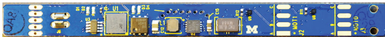
Figure 3.13: Electronics driver board for the fiber positioner, which was laid out at University of Michigan. On the left side is the spring clip which retains the fiber. On the right the two holes are where the board screws to the aft end of the positioner. The board is 8 mm wide and has been carefully designed so that all components, connectors, and fiber pass easily through the focal plate interface.
