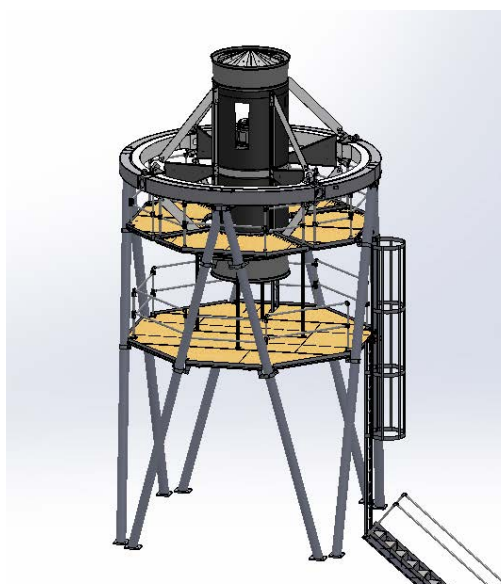
Figure 8.6: Preliminary design for both upper and lower top end platforms, showing access ladder and stairs, and showing upper platform supported by upper truss braces.
