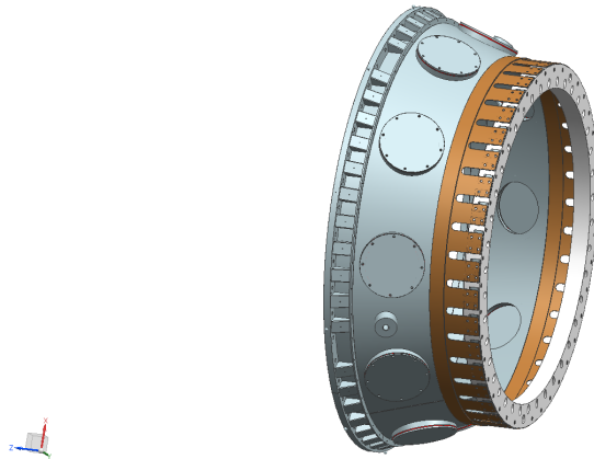
Figure 2.17: This picture shows the Focal Plane Adaptor or FPD. The left side attaches to the barrel and the right side to the Focal Plane Assembly.
