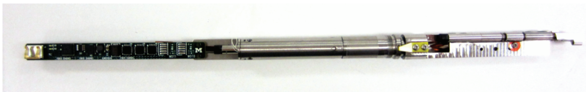
Figure 3.8: Prototype of the DESI 10.4 mm pitch fiber positioner.
