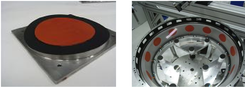
Figure 2.8: Mounting of the DECam optics. Shown at left is a pad and insert, and at right the radial and axial pads attached to the lens.
