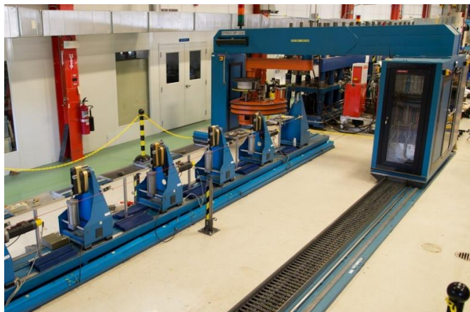
Fig. 1a. Spirex Selva coil winding machine
