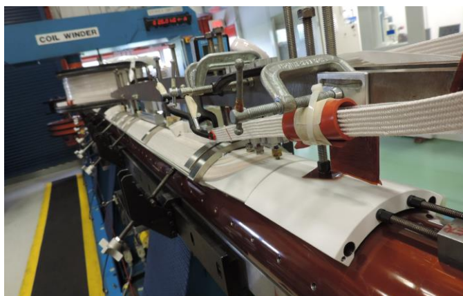
Fig. 1b. Completed inner layer coil with outer layer conductor fastened on top
