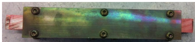
Fig. 3: Bare cable stack in its reaction fixture.
