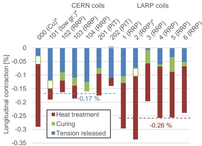
Fig. 7: Longitudinal contraction of MQXF CERN and LARP coils [13], after tension release, curing and heat treatment. The average total contraction is indicated on the plot. \*For these coils, no data were available on the contraction during curing. A contraction of  $-0.03\%$  is then assumed (open bars), the total being conserved.
