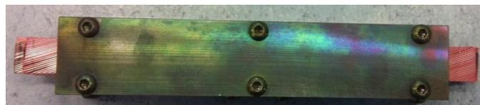
Fig. 3: Bare cable stack in its reaction fixture.
