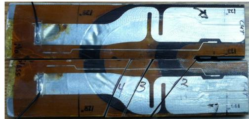
Fig. 4 HQ03 Coil Return End Autopsy
