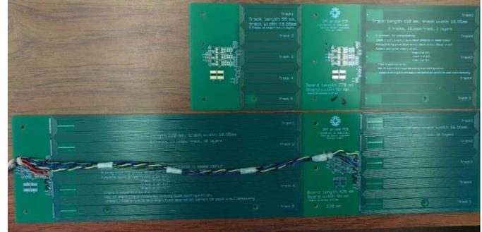
Fig. 1 Circuit board probes used for the measurements. Top: the 55 mm/110 mm 2-layer PCB; bottom: the 220 mm/110 mm 30-layer PCB.
