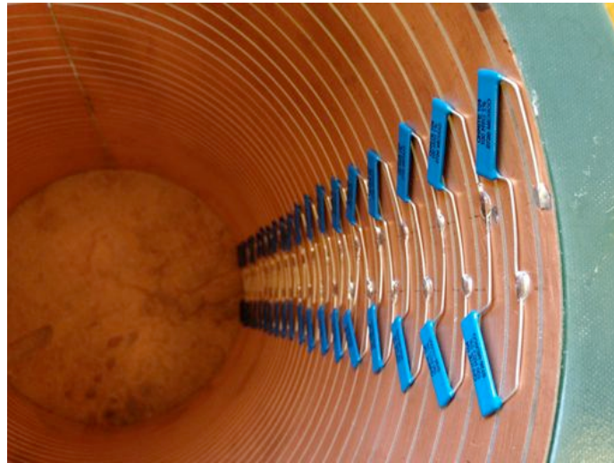
Figure 2: One chain of the resistors soldered to the inner surface of the copper sheet.
