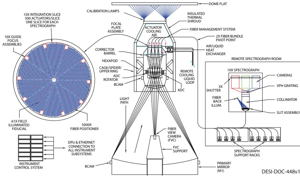
Figure 5. Block diagram of the DESI system. The focal plane is divided into petals that each contain 500 fiber positioners and a guide and focus sensor. The fibers for each petal are bundled into a jacketed cable and then routed down the telescope to a three armed spectrograph located in the Coudé room
