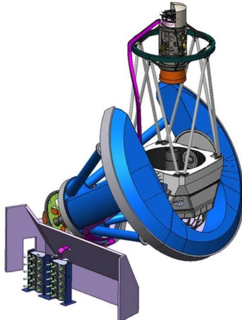
Figure 1. DESI on the Mayall telescope. The 5000 fiber positioner is located at the top of the prime focus cage under the cap (grey). The fiber bundles (purple) will cross the optical path in the shadow of the the support fins and be routed around the declination and polar axes allowing for telescope motions and then terminating at the spectrographs in the code room.
