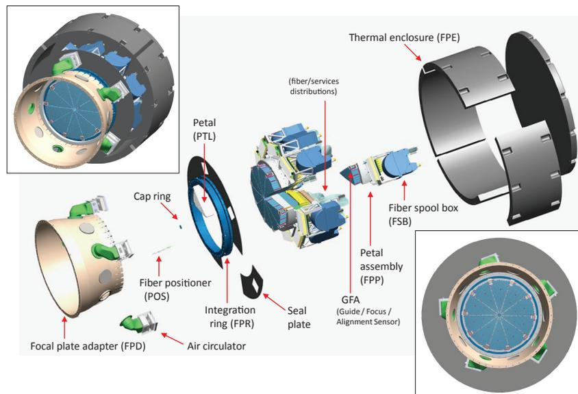
Figure 7. DESI focal plane system.
