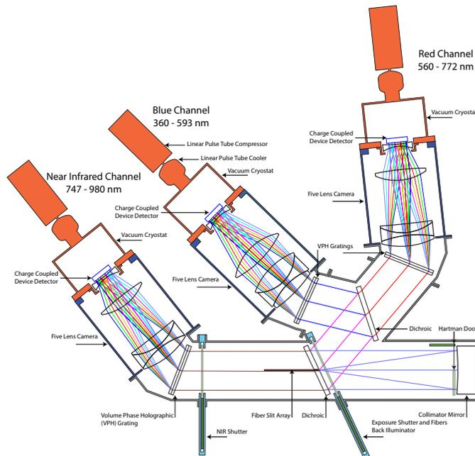
Figure 9. DESI three channel spectrograph
