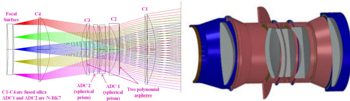
Figure 6. Left: DESI final optical design. the largest lens, C1, is 1.14m in diameter and the total mass of the lenses in the design is 863kg. The two smaller fused silica lenses have aspheric surfaces on one face, with all other silica surfaces spherical. Right: Optical elements assembled into the corrector barrel.
