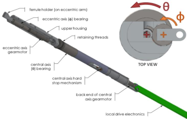
Figure 8. DESI theta-phi actuator.
