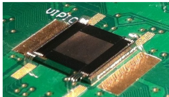
Fig. 5. Picture of a VIPIC1 die that was thinned from a side of the upper tier mounted on a PCB for bench tests.
