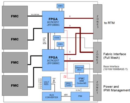
**Figure 2.** The Pulsar IIa block diagram.
