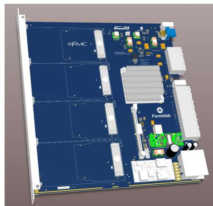
**Figure 5.** The Pulsar IIb board in layout.
