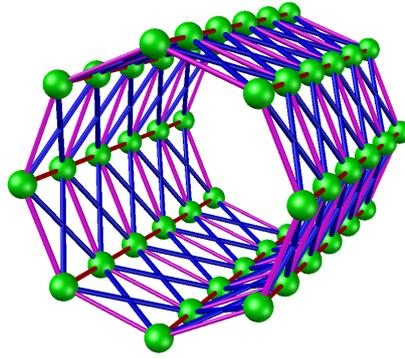
**Figure 1.** Conceptual view of a proposed CMS phase 2 Level-1 tracking trigger which consists of 48 towers ( $6\eta \times 8\phi$ ). Trigger tower processor crates (shown in green) share data with immediate neighbors only.
